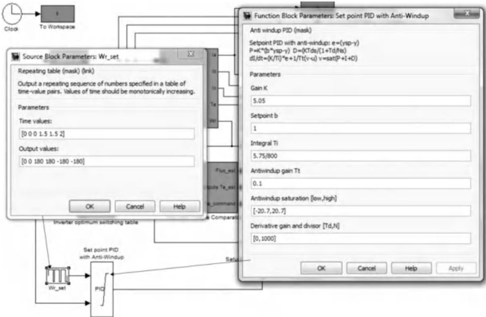
Figure 5.107 Speed command and parameters of PID controller
