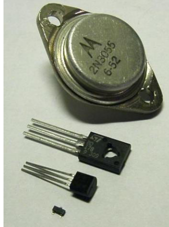
Assorted discrete transistors. Packages in order from top to bottom: TO-3, TO-18, TO-92, SOT-23.
