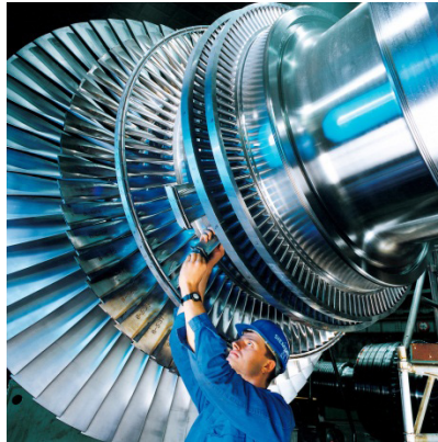
Rotor of a modern steam turbine, used in a power station.
