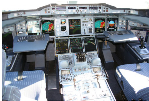
The Airbus A380 glass cockpit featuring pull-out keyboards and two wide computer screens on the sides for pilots.
