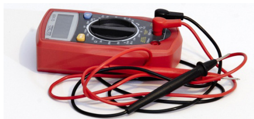
A multimeter can be used to measure the voltage between two positions.
