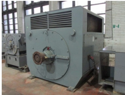
Large 4,500 HP AC Induction Motor.
