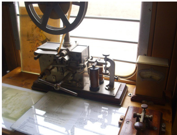
A printing electrical telegraph receiver, with transmitter key at bottom right
