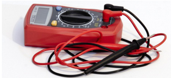
A multimeter can be used to measure resistance in ohms, among other things.
