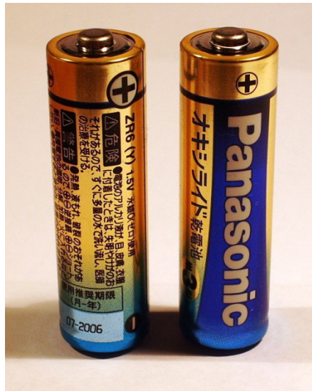
A pair of AA cells. The + sign indicates the polarity of the potential difference between the battery terminals.
