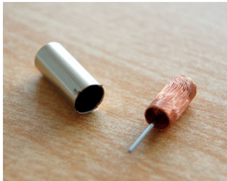
A miniature coreless motor
