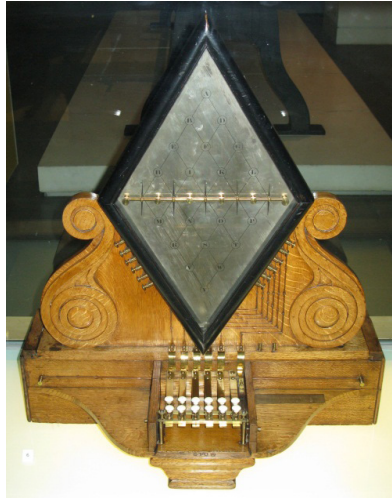
Cooke and Wheatstone's five-needle, six-wire telegraph
