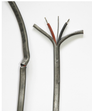
Lead cased electrical wire from a circa 1912 house in Southern England. Two conductors are sheathed in red and black rubber, the central earth wire is bare. These wires are dangerous because the sheath is prone to split if repeatedly flexed.
