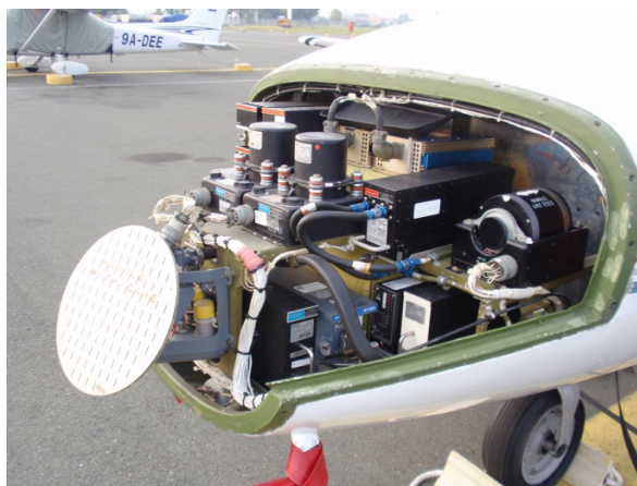
Radar and other avionics in the nose of a Cessna Citation I/SP
