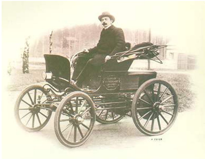
Figure 2. First EV,s were possible to cross up to 100 km, moving with speed below 20 km/h.
