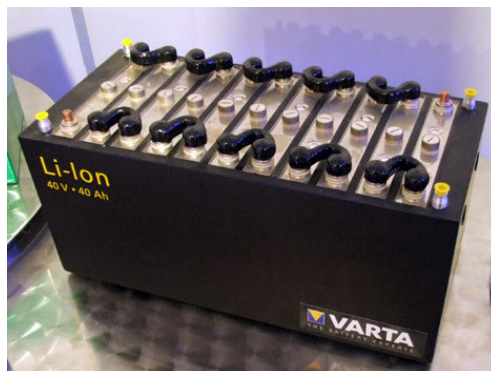
Figure 22. A typical Li-ion battery pack utilized in the EVs [21].
