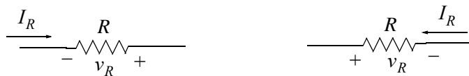
Figure 2.3. Voltage polarity and current direction not in accordance to passive sign convention
