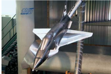
Fig. 1. X-31 Remote control model in the DNW-NWB Braunschweig.
