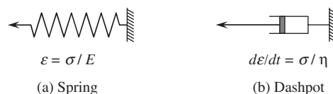
Figure 5-52 Spring and dashpot for modeling viscoelastic behavior
