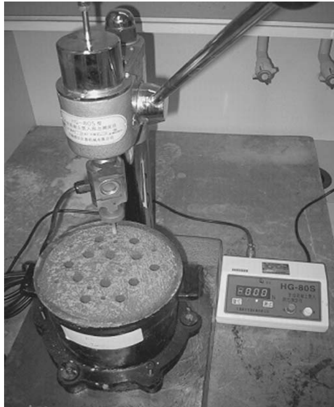
Figure 3-8 Measurement setup of concrete mixture setting time
