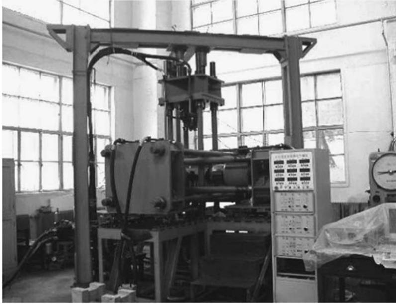
Figure 5-16 Triaxial testing machine at Dalian University of Technology
