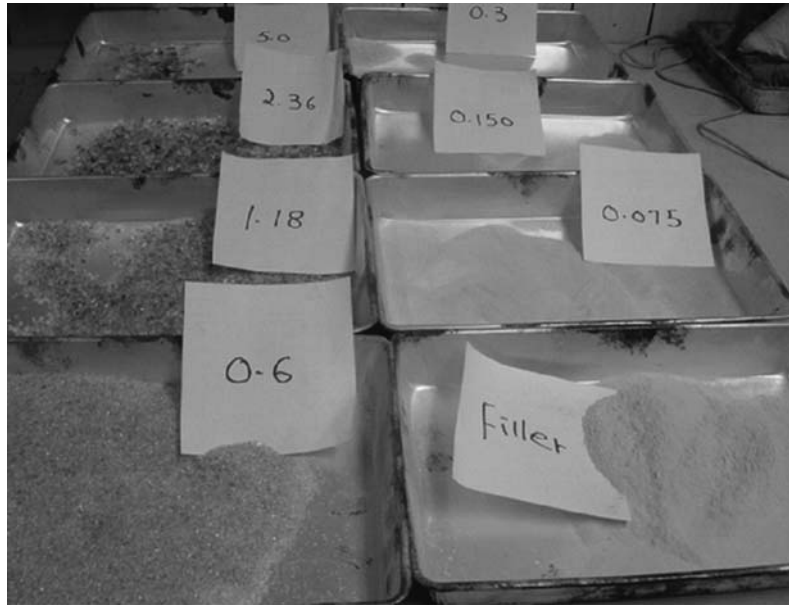
Figure 9-1 Recycled waste glass as an aggregate for concrete
