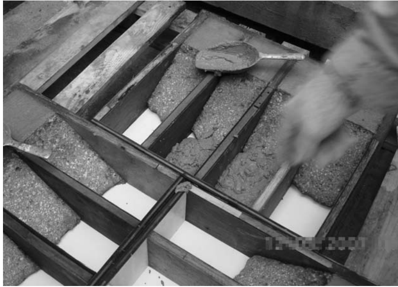
Figure 6-38 Casting of prisms for slant shear measurement
