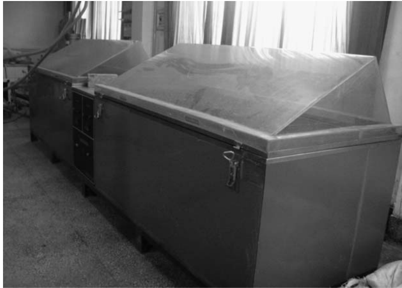
Figure 5-77 Seawater tank for marine environmental simulation test
