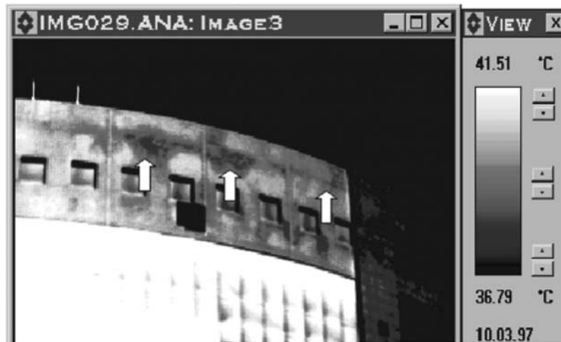
Figure 8-49 The lower-temperature areas (indexed by upward arrows) indicating the defected areas filled with water or moisture
