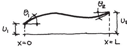
Fig. 13.29 Prescribed boundary conditions for the general beam element
