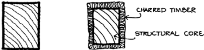
Fig. 5.38 Timber before and after burning
