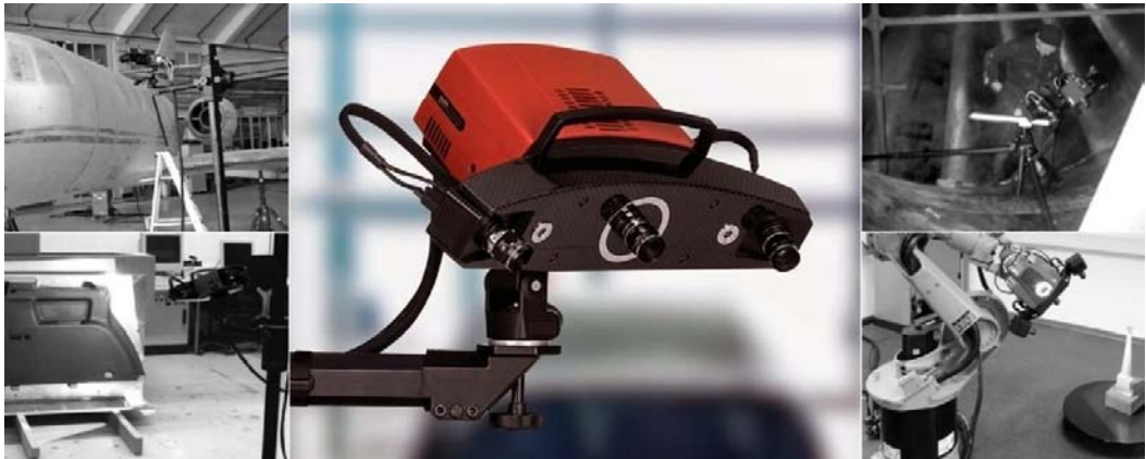
Figure 8. ATOS III general purpose structured light scanner.
