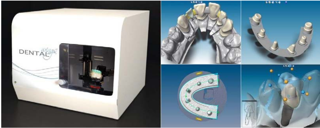
Figure 7. DentalWings laser scanner for dental applications.
