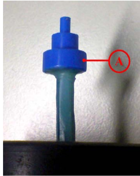
Figure 2. The wax pattern and the location where the thermocouple has been placed (point A).
