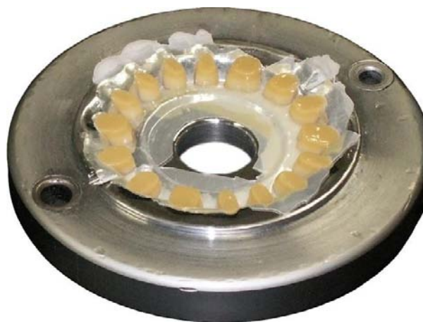
Figure 2. Final mold and molded sets of acrylic teeth with flash.
