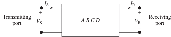
FIGURE 9.25 Two-port representation of transmission line.
