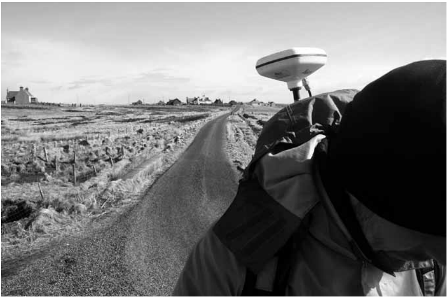
Figure 3.4 NALS surveyor with dGPS enroute between sites in the townships of Ness
