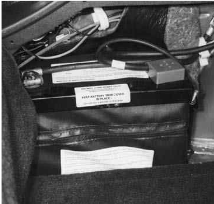
Figure 7-9. This Ford Escort diesel battery is encased in a protective bag and housed in the trunk.
