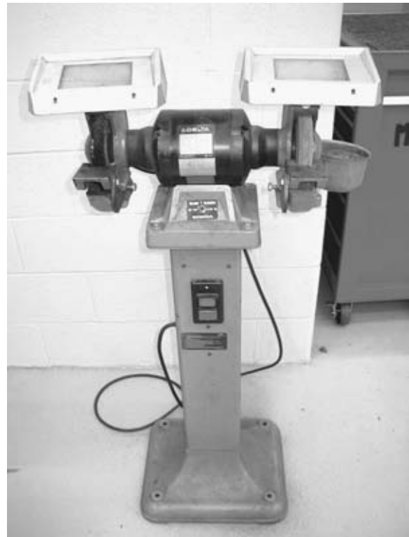
Figure 1-22. Pedestal grinder with shields. This type of grinder should be bolted to the floor. A face shield should also be worn whenever using a grinder or wire wheel.
