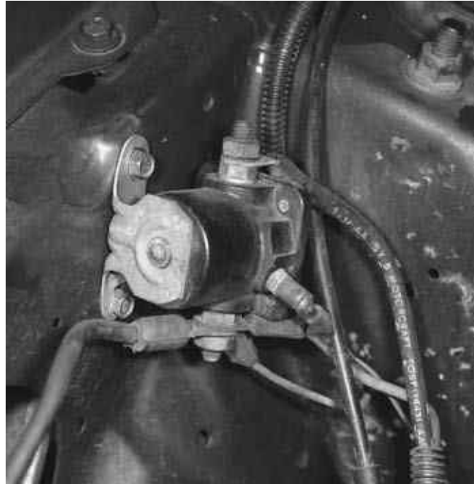
Figure 9-12. The Ford starter relay or magnetic switch.
