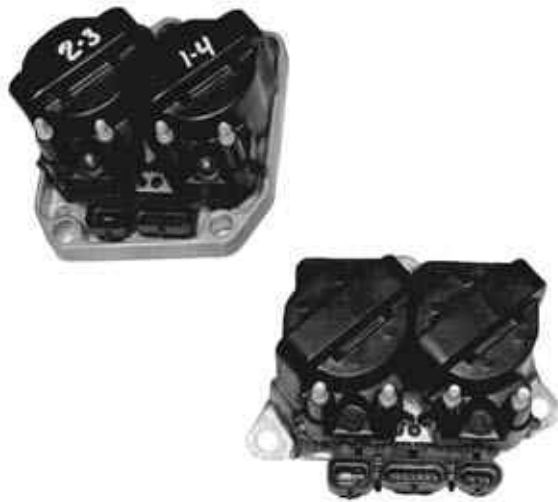
Figure 11-29. Typical DIS coil packs used on cylinder engines.
