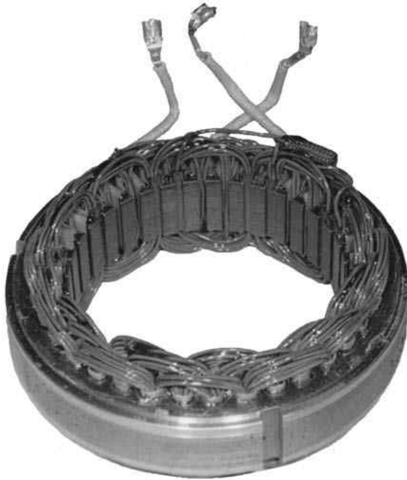
Figure 8-14. An AC generator (alternator) stator.
