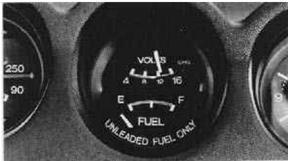
Figure 8-52. Automotive voltmeter in instrument panel.
