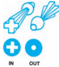
Figure 4-9. Current direction symbols.
