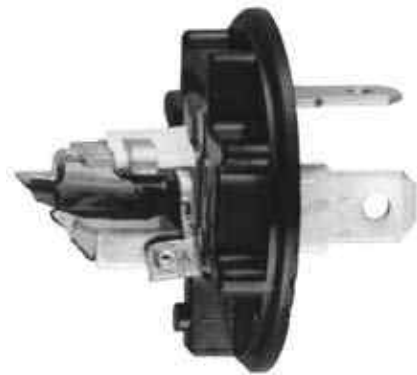
Figure 12-39. The internal components of a turn signal flasher.
