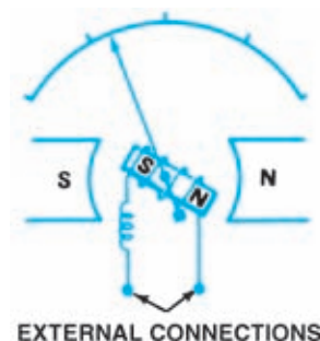
Figure 13-2. The D'Arsonval movement uses the field interaction of a permanent magnet and an electromagnet.
