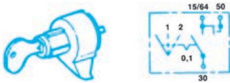
Figure 9-2. This ignition switch acts directly on the contact points. (Reprinted by permission of Robert Bosch GmbH)
