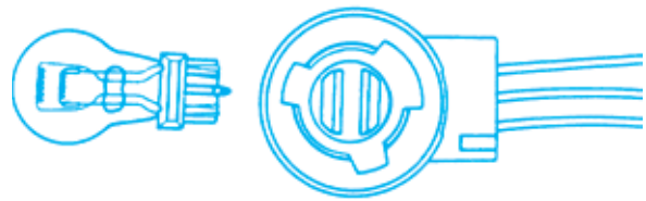
Figure 12-30. Wedge-base bulbs with plastic sockets are used for some external lighting applications. (DaimlerChrysler Corporation)
