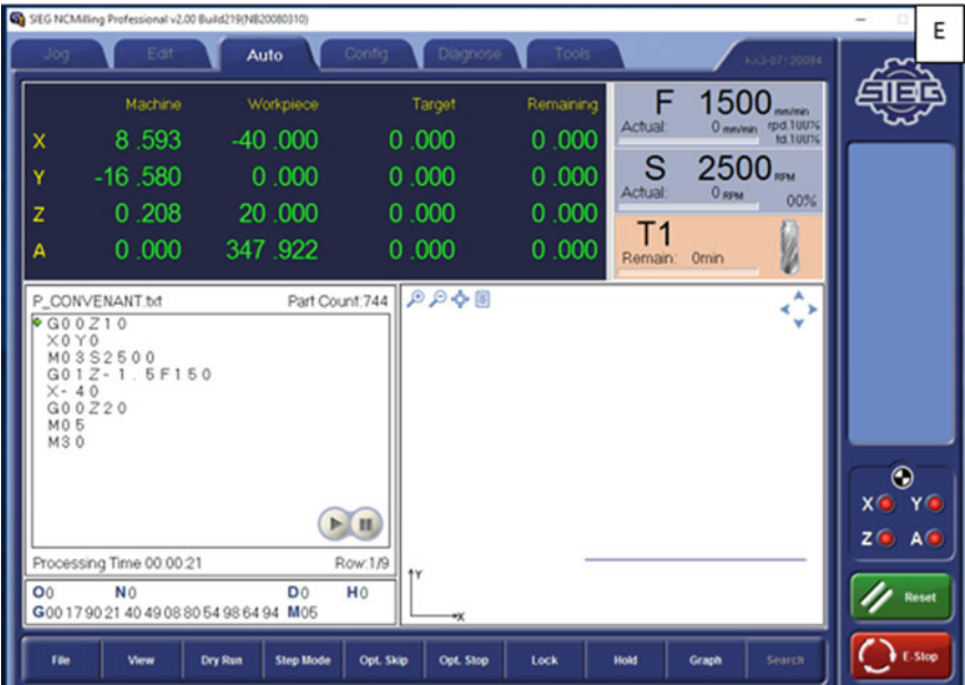
Appendix A–E: The CNC programming language software employed for various machining parameters during operations
