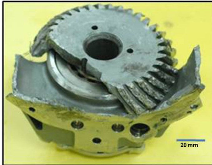
FIGURE 10.2 Fractured bevel pinion in the housing.
