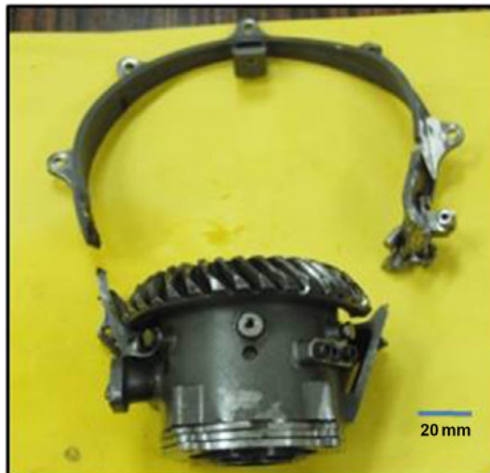
FIGURE 10.3 Photograph of the pinion housing after the failure.
