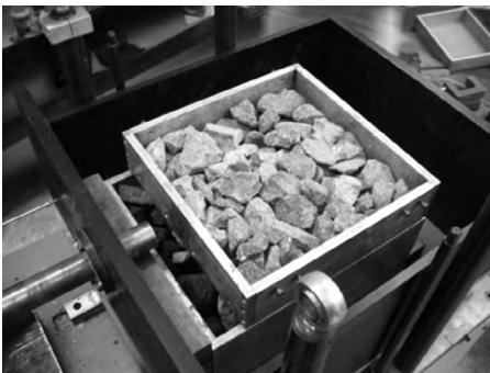
Figure 3.12 Large direct shear apparatus. (Courtesy of University of Illinois Urbana-Champaign, Champaign, Illinois.)
