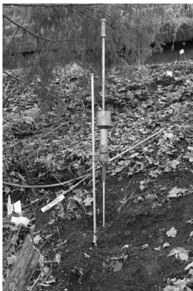
Figure 7.16 Dynamic Cone Penetrometer (DCP) on slope.
