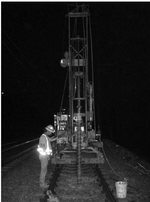
Figure 8.6 Soil drilling in the gauge of the track using a hollow stem auger.
