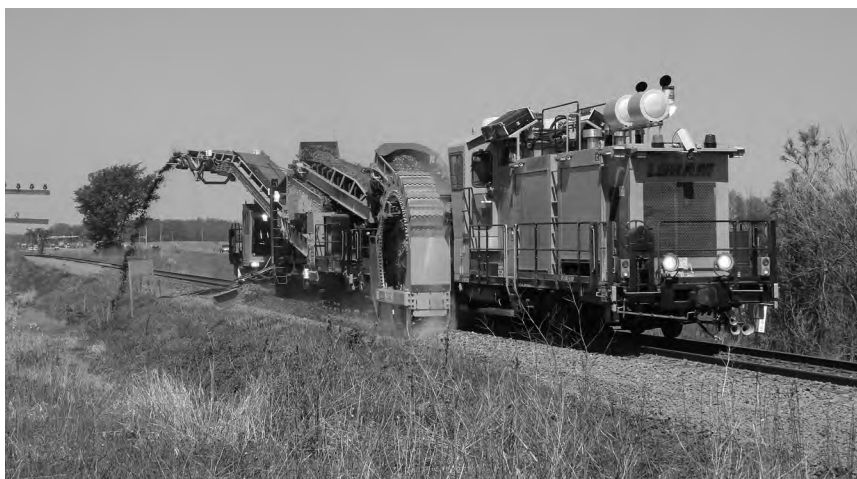
Figure 6.43 Picture of a shoulder cleaner. (Courtesy of Loram Maintenance of Way, Hamel, Minnesota.)
