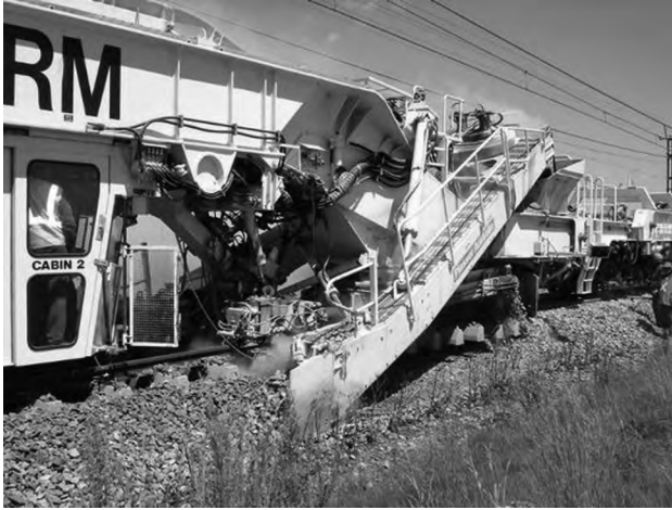
Figure 6.44 Excavating chain of ballast undercutter. (Courtesy of R. Wenty, Plasser & Theurer, Vienna, Austria.)
