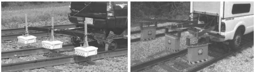
Figure 8.16 Three 400 MHz antennas installed on a hyrail vehicle (left photo). Three 2-GHz antennas on a hyrail vehicle (right photo).
