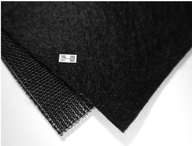
Figure 6.24 Examples of woven and nonwoven geotextiles.
