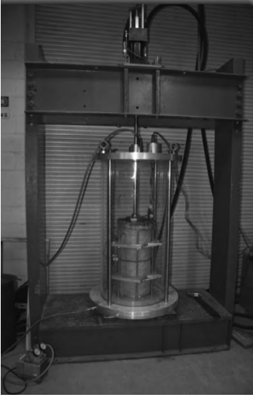
Figure 3.13 Large (0.3 m, 12 in. diameter) triaxial test apparatus. (Courtesy of University of Illinois Urbana-Champaign, Champaign, Illinois.)
