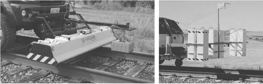
Figure 8.14 Hyrail-based GPR system, showing a single 400 MHz antenna and 3D-radar system (left photo), and three pairs of 1-GHz horn antennas (right photo).
