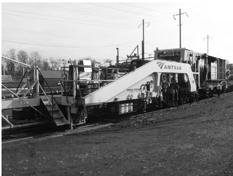
Figure 1.32 Tamping machine for track surfacing and alignment.
