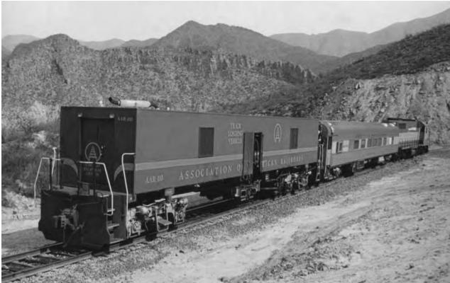
Figure 8.53 TTCI's Track Loading Vehicle (TLV). (Courtesy of Transportation Technology Center Inc., Pueblo, Colorado.)
