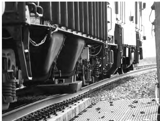
Figure 1.29 Loaded profile at bridge transition.
