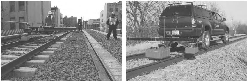
Figure 8.15 Push-cart application of railway GPR (left photo) and 200 MHz (left) and 400 MHz (right) GPR antennas installed on the back of a hyrail vehicle (right photo).
