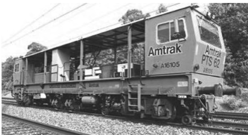
Figure 1.33 Dynamic track stabilizer.
