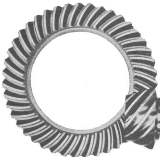
Figure 7.39 Hypoid bevel gear. Reproduced from Mabie and Reinholtz, Mechanisms and Dynamics of Machinery , 4th edition, John Wiley & Sons, © 1987
