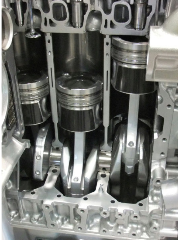
Figure 13.28 Partial cross-sectional view of an internal combustion engine
