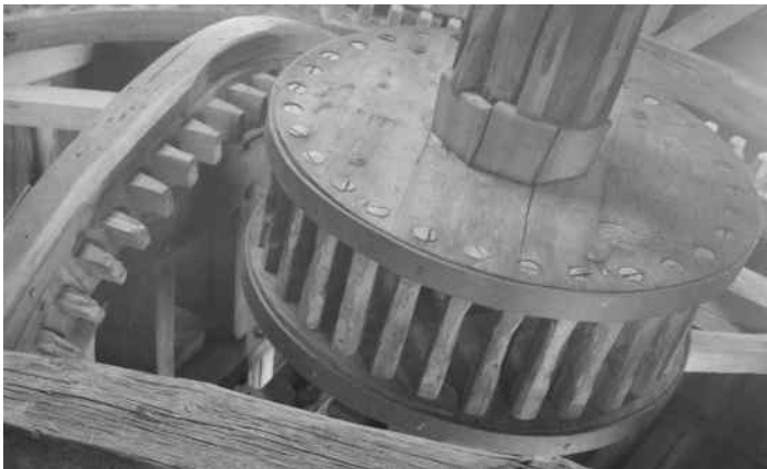
Figure 7.2 Cage gear from Pantigo Windmill, Long Island, New York
