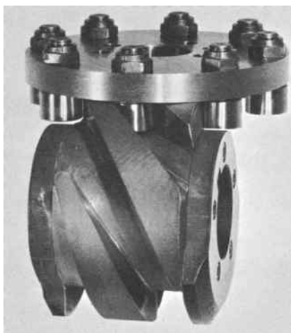
Figure 9.1 Cylindrical cam indexing drive. Reproduced from Tuttle, Mechanisms for Engineering Design , John Wiley & Sons, © 1967
