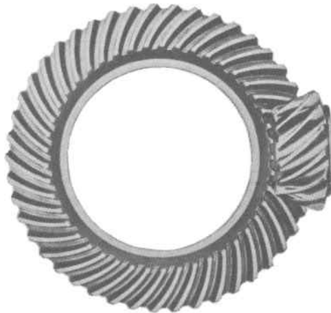
Figure 7.38 Spiral bevel gear. Reproduced from Mabie and Reinholtz, Mechanisms and Dynamics of Machinery , 4th edition, John Wiley & Sons, © 1987
