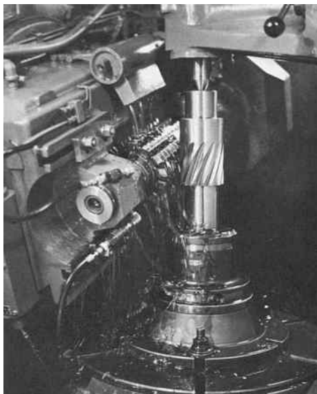
Figure 1.30 Hobbing a helical gear. Reproduced from Mabie and Reinholtz, Mechanisms and Dynamics of Machinery , 4th edition, John Wiley & Sons, © 1987
