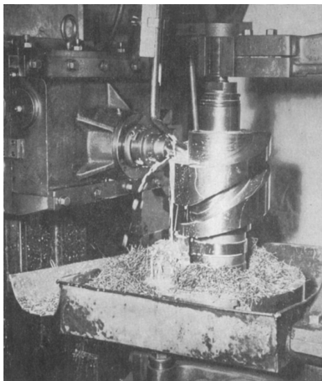
Figure 1.37 Cutting a cylindrical cam
