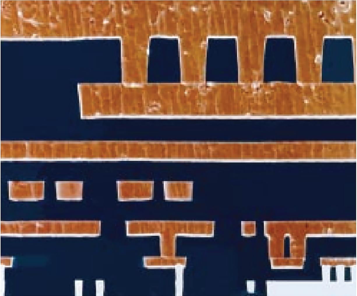
Figure 18.19 Cross section of a six-level copper wiring structure fabricated by IBM.
