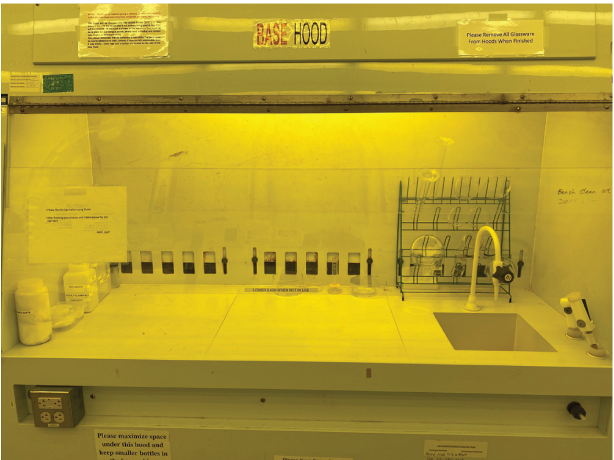
Figure 14.2 A fume hood with simple structure for wafer cleaning, wet etching, and developing.
