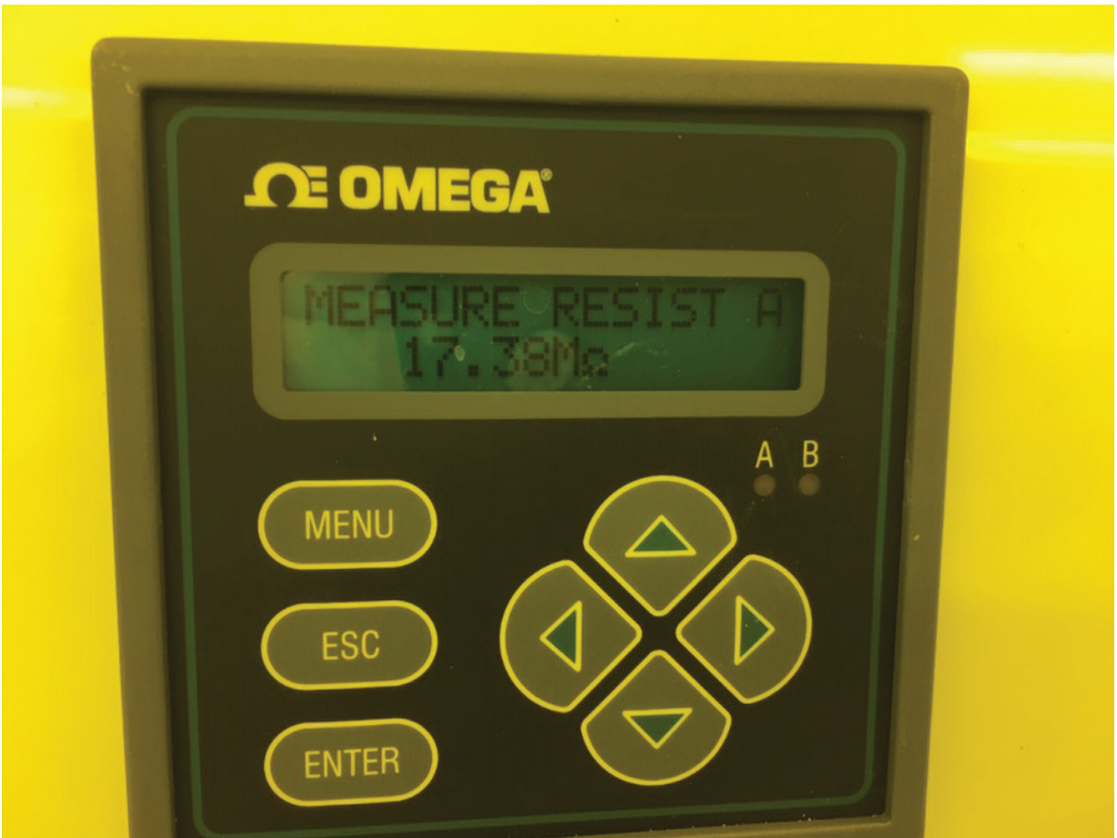
Figure 7.14 The resistivity of DI water with the unit of \text{M}\Omega\cdot\text{cm} .
