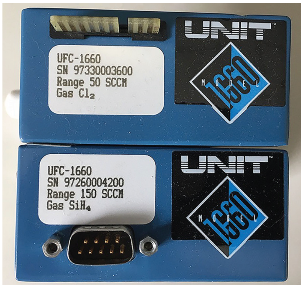
Figure 14.19 \text{Cl}_2 , 50 sccm MFC and \text{SiH}_4 , 150 sccm MFC.
