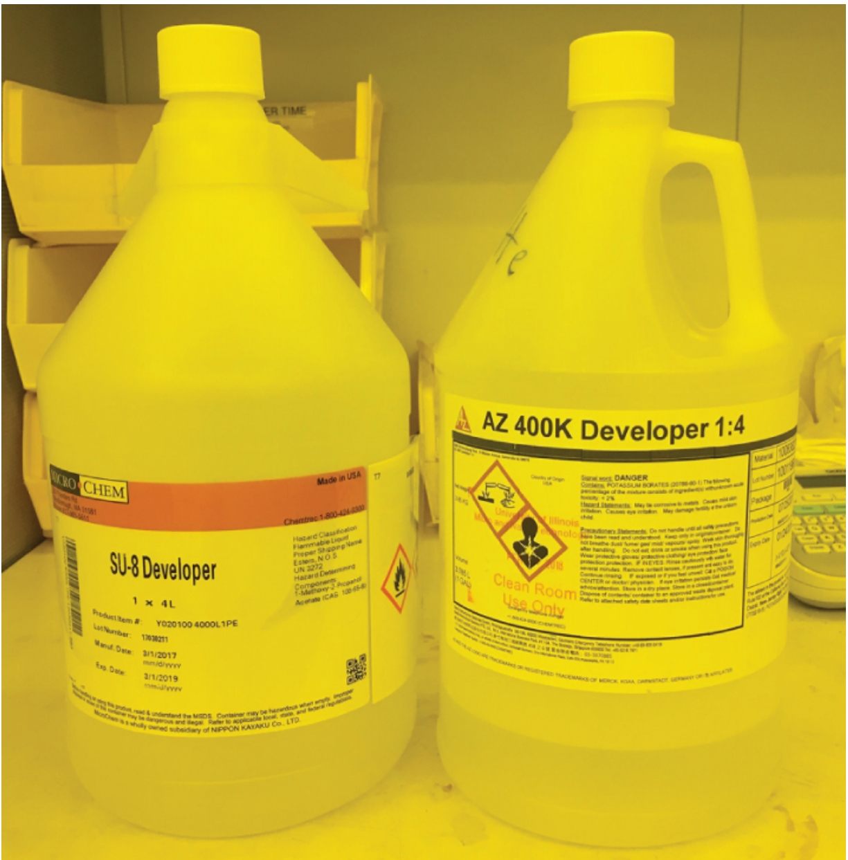
Figure 12.15 Negative PR developer (left) and positive PR developer (right).
