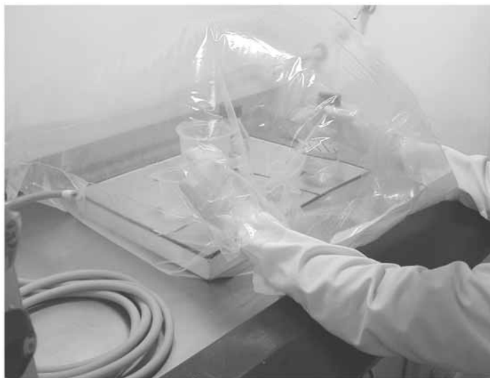
Fig. 1. A researcher performing an EMS mutagenesis experiment inside an Atmos bag purchased from Aldrich. All equipment needed is inside the Atmos bag. The researcher is wearing full protective clothing, including two pairs of gloves.
