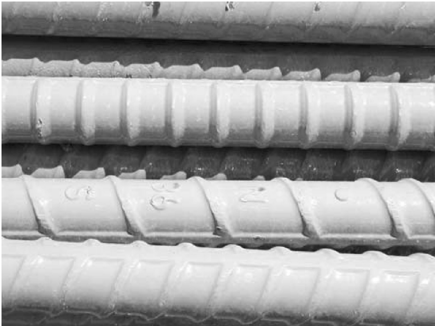
Figure 4.24 Damages and scratches on the epoxy coating of new steel bars.
