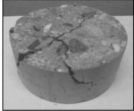
Figure 4.18 Concrete specimens exposed to maximum temperature 800 °C and cooled down by natural cooling.
