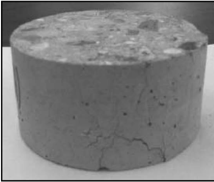
Figure 4.18 Concrete specimens exposed to maximum temperature 800 °C and cooled down by natural cooling.
