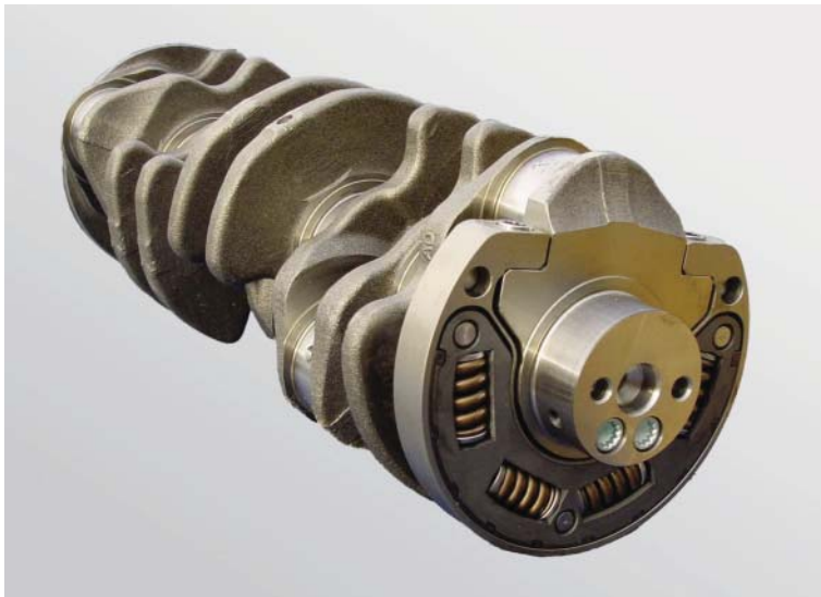
Figure 9.28 Internal crankshaft damper (reproduced with permissions of Schaeffler)
