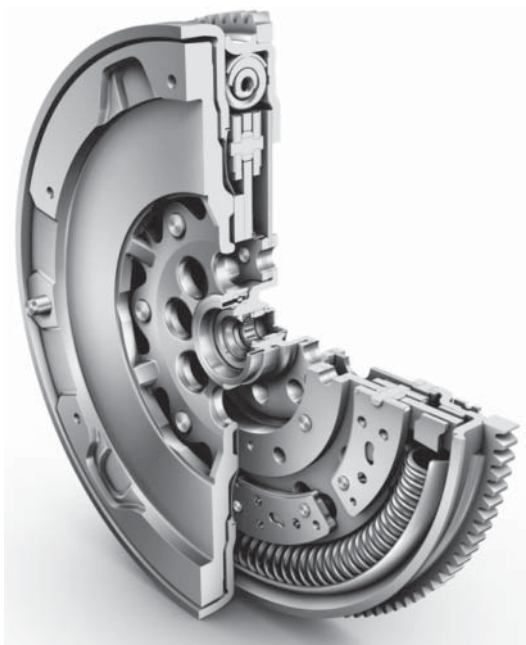
Figure 17.8 Dual-mass flywheel with centrifugal pendulum absorber (reproduced with permissions of Schaeffler)
