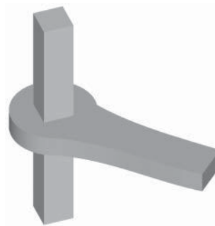
Figure 20.4 Translational joint or prismatic joint
