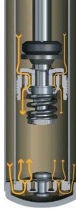
Figure 18.6 Twin-tube shock absorber: details of flow for rebound (reproduced with permissions of ZF Friedrichshafen AG)
