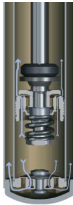
Figure 18.5 Twin-tube shock absorber: details of flow for compression (reproduced with permissions of ZF Friedrichshafen AG)
