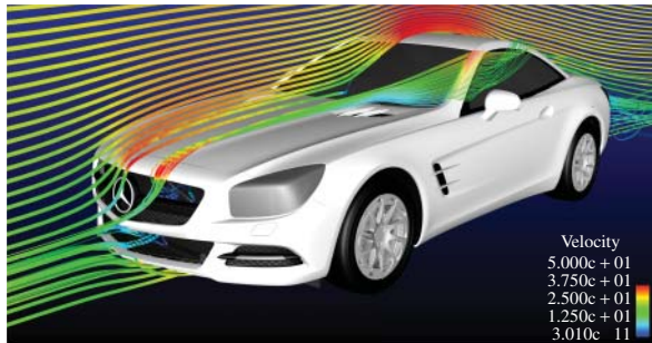
Figure 3.3 Vortex at engine compartment and at A-column (reproduced with permissions of Daimler AG)
