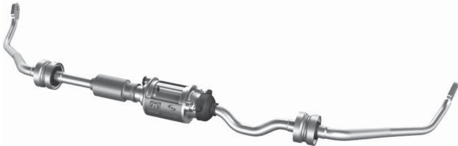
Figure 14.9 Active roll stabilization (ARS): active anti-roll bar (reproduced with permissions of ZF Friedrichshafen AG)
