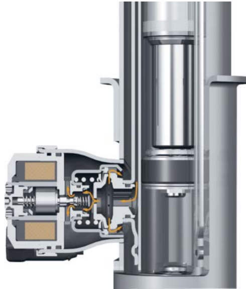
Figure 18.7 Proportional valve in a CDC (reproduced with permissions of ZF Friedrichshafen AG)
