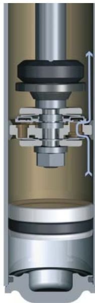
Figure 18.2 Monotube shock absorber: details of flow for compression (reproduced with permissions of ZF Friedrichshafen AG)
