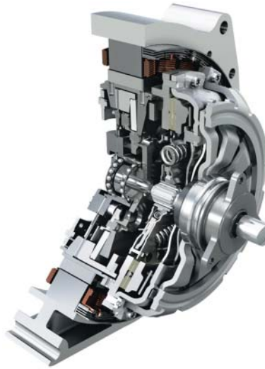
Figure 7.4 Electric engine integrated in the powertrain (reproduced with permissions of Schaeffler)
