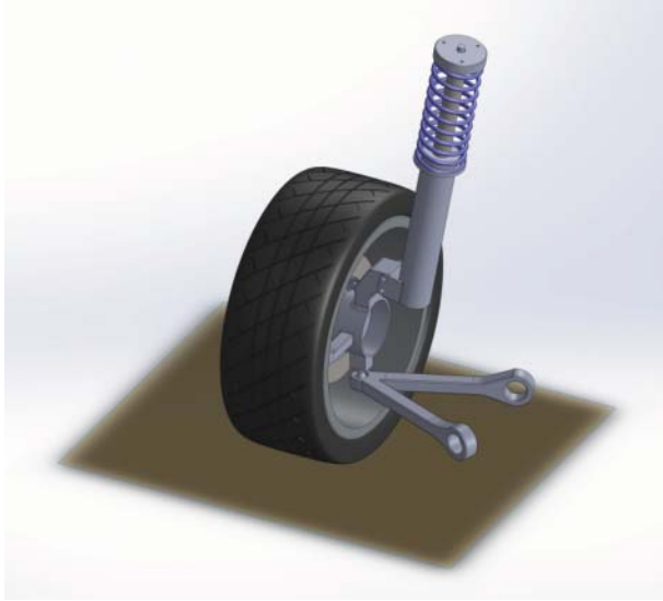
Figure 16.6 Principal components of a McPherson front axle suspension
