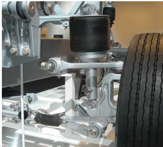
Figure 18.19 Air spring in a truck wheel suspension (reproduced with permissions of ZF Friedrichshafen AG)
