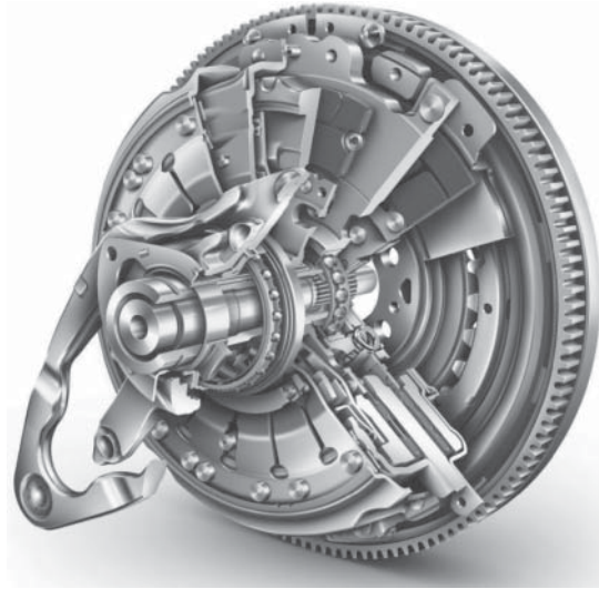
Figure 17.1 Dual dry clutch (reproduced with permissions of Schaeffler)
