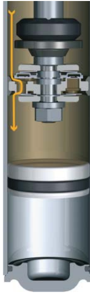
Figure 18.3 Monotube shock absorber: details of flow for rebound (reproduced with permissions of ZF Friedrichshafen AG)
