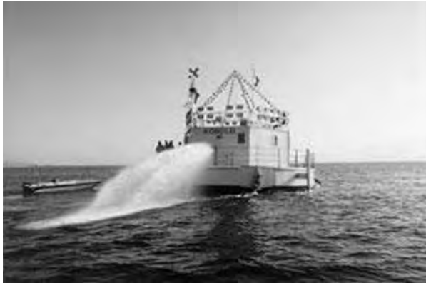
Figure 10.3 Enermar: Kobold turbines, Messina, Italy (prototype 40kW) Source: Ponte di Archimede International S.p.A.
