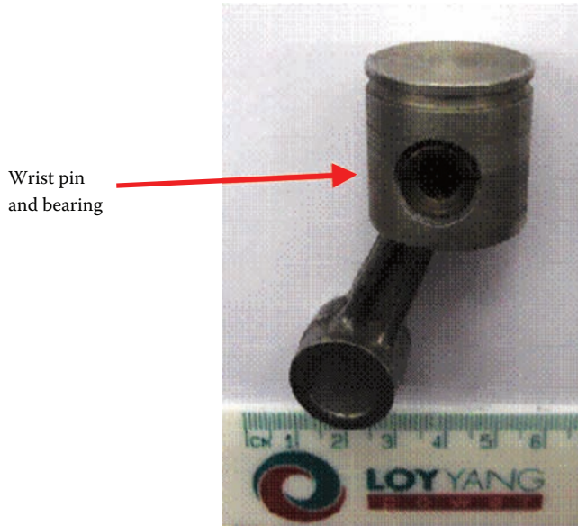
FIGURE 2.25 Piston and connecting rod of a small reciprocating compressor.
