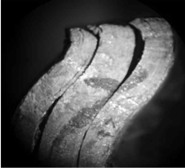
14.3 Delamination of compression specimen during testing.
