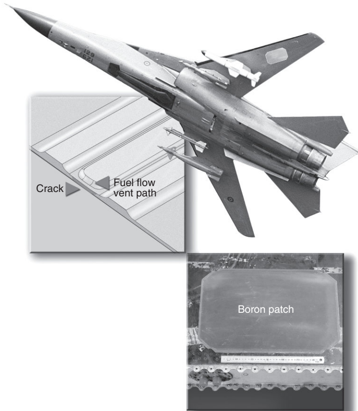
2.19 Region of fatigue cracking in F-111 lower wing skin and, inset, a photograph of the boron/epoxy repair.
