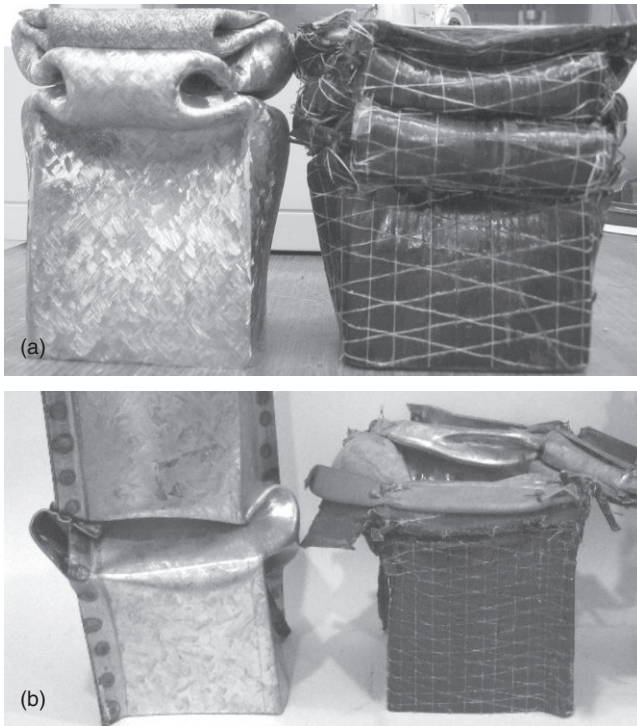
6.5 Typical quasi-static axial crushing mechanisms: (a) 75 × 75 × 2 SHS; (b) 100 × 100 × 1.66 mm SW SHS (Bambach and Elchalakani, 2007; Bambach et al. , 2009c).
