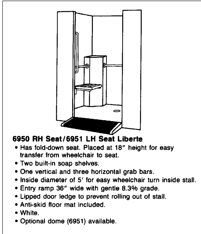
FIGURE 10.12 ■ Handicap shower with seat and ramp. (Courtesy of McGraw-Hill)
