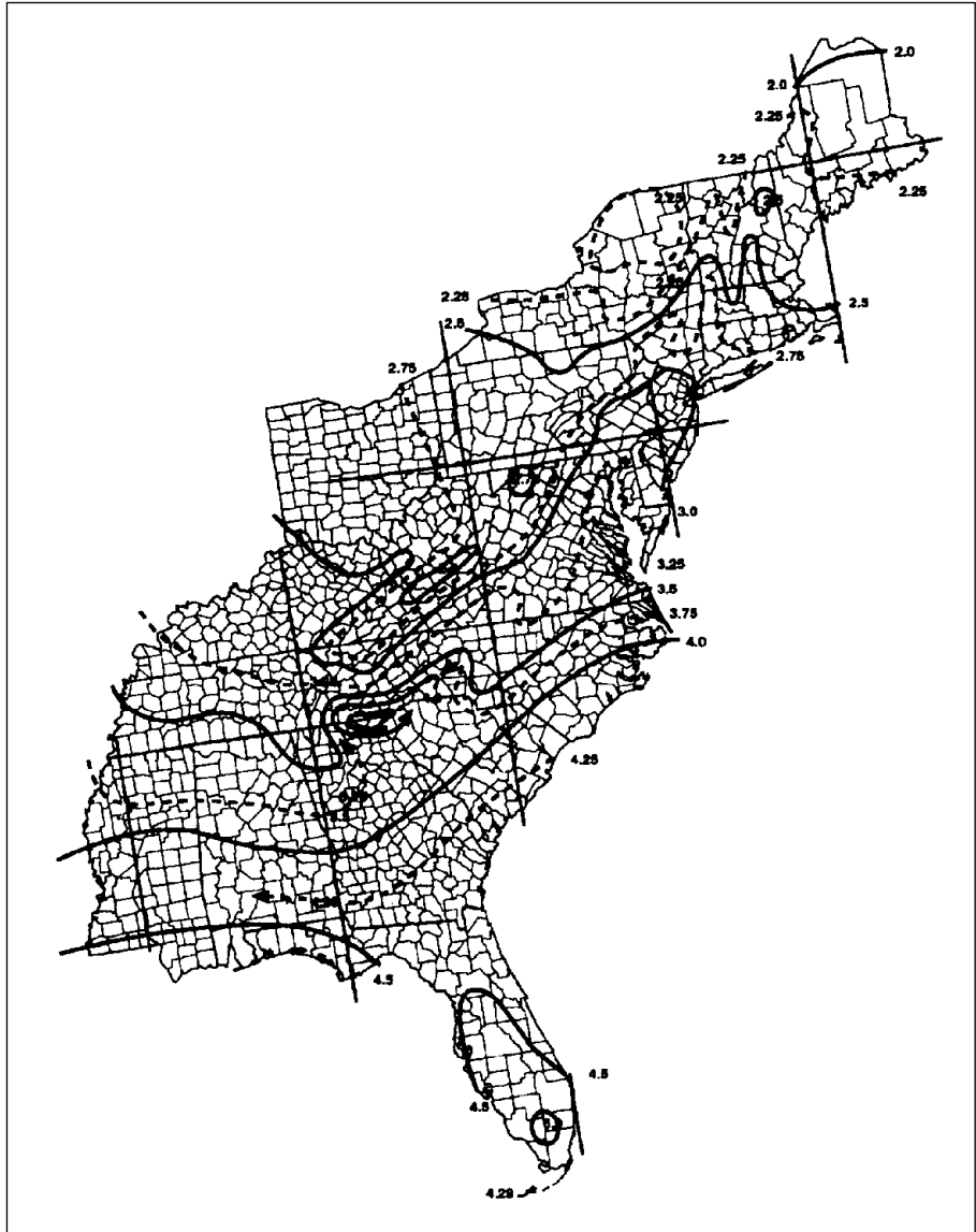
FIGURE 13.44 ■ 100-year, one-hour rainfall rate for the eastern United States. (Courtesy of International Code Council, Inc. and the International Plumbing Code 2000)
