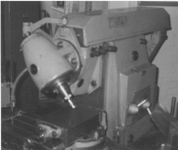
Vertical milling attachment fitted to a horizontal milling machine
