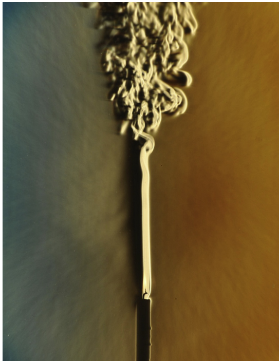
Figure 5.7 Laminar, transitional, and turbulent flow above a candle. (By Gary Settles—Own work, CC BY-SA 3.0, https://commons.wikimedia.org/w/index.php?curid=29522249 .)
