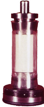
Figure 4.6 Rock sample ready for compression testing at downhole conditions. Courtesy: IADC.
