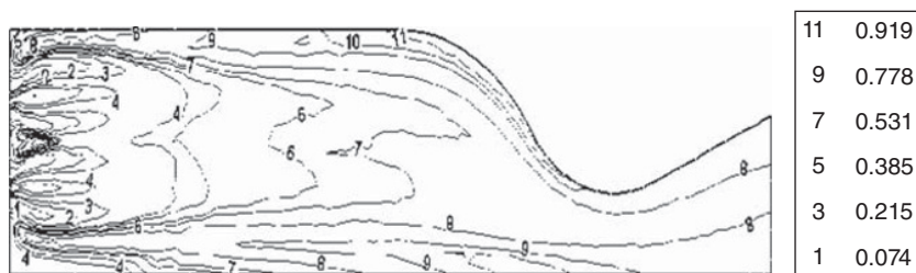
Figure 8.9 Mol. coefficient profile of H 2 O for oxidant-rich condition, centrifugal injector.
