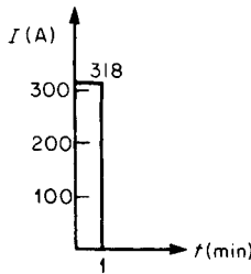
FIGURE 18.12 Load profile for the first minute.
