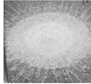
Fig. 11.6.39 Rear wall after impact.
