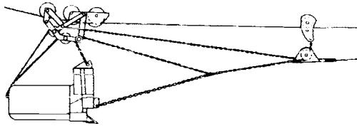
Fig. 10.4.43 Slackline-cable bucket and trolley.
