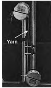
Fig. 20.10.2 Yarn tensile testing using Instron textile grips.
