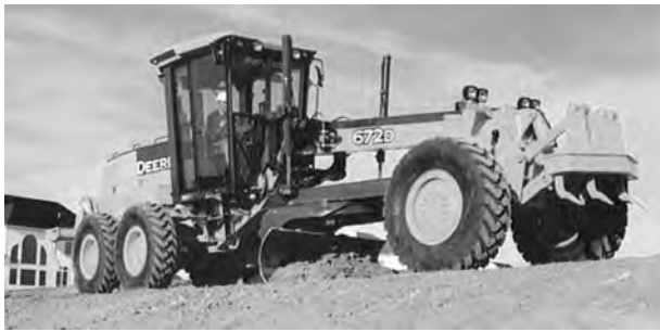
Fig. 10.4.10 Six-wheel articulated-frame motor grader. (John Deere.)
