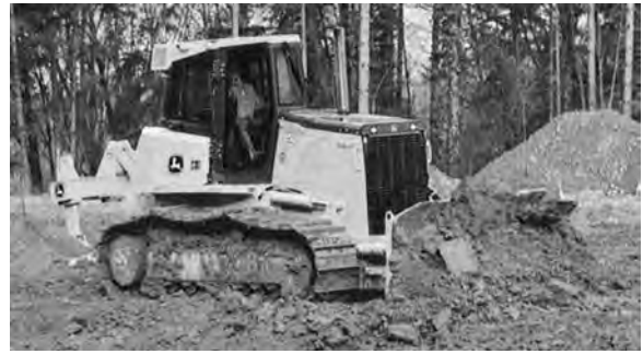
Fig. 10.4.4 Crawler tractor with dozer blade. (John Deere.)
