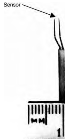
Fig. 20.7.6 Photograph of boundary-layer-type hot-wire probe.
