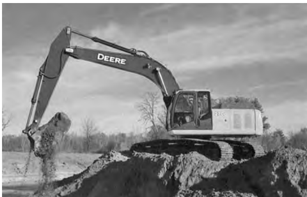
Fig. 10.4.11 Excavator with tracked undercarriage. (John Deere.)
