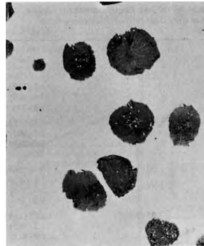
Fig. 6.3.4 Ductile iron with spherulitic graphite. Unetched, 100 X.
