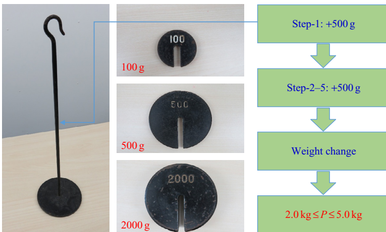
Fig. 8.17 Loading methods and test procedure.
