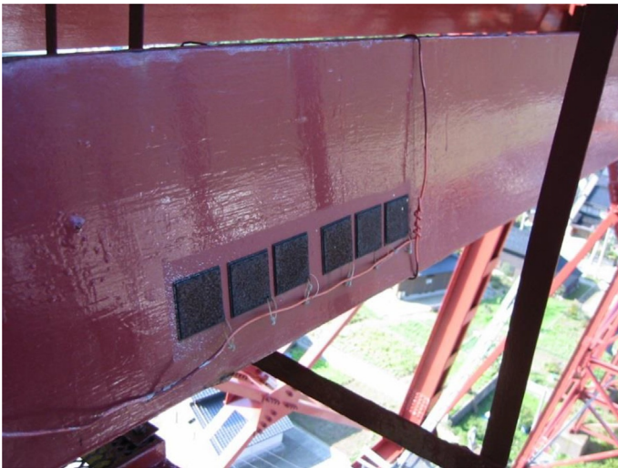
Fig. 13.5 Monitoring of corrosion environment due to sea breeze. (Photo by Yoda.)
