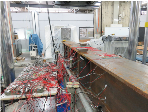
Fig. 7.21 Steel-concrete composite beams under combined negative bending and torsional moments.
