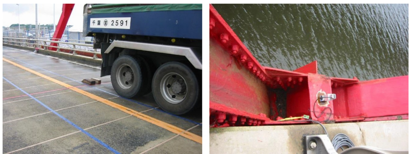
Fig. 13.4 Vibration test of a Truss Bridge. (Photos by Yoda.)
