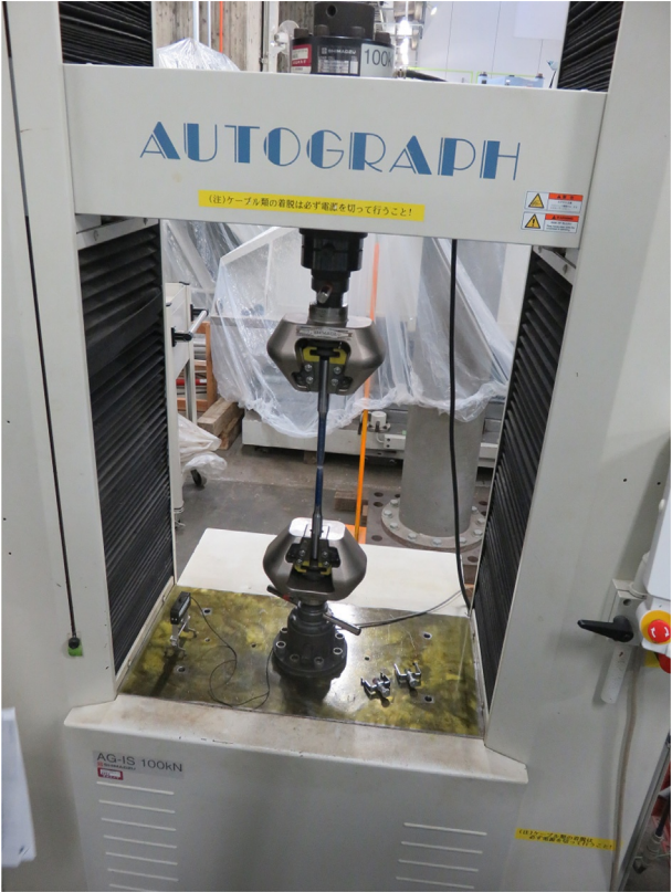
Fig. 3.5 Tensile test for steel. (Photo by Lin.)
