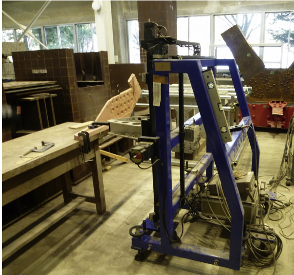
Fig. 14.4 Metal thickness measurement device with laser displacement sensors. (Photos by LIN.)
