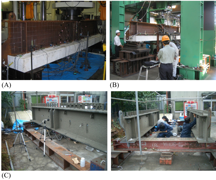
Fig. 7.17 Static test, fatigue test, and impact test set-up. (A) Static loading test. (B) Fatigue loading test. (C) Impact test.
