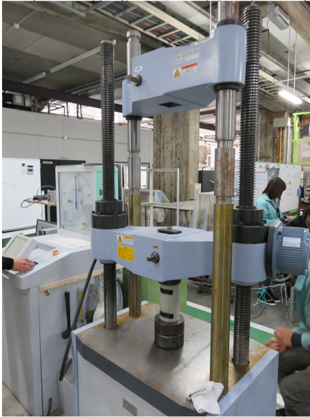
Fig. 3.7 Compression test for concrete. (Photo by Lin.)
