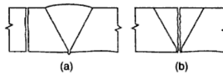
Fig. 3.15 Failure of Butt Welds
