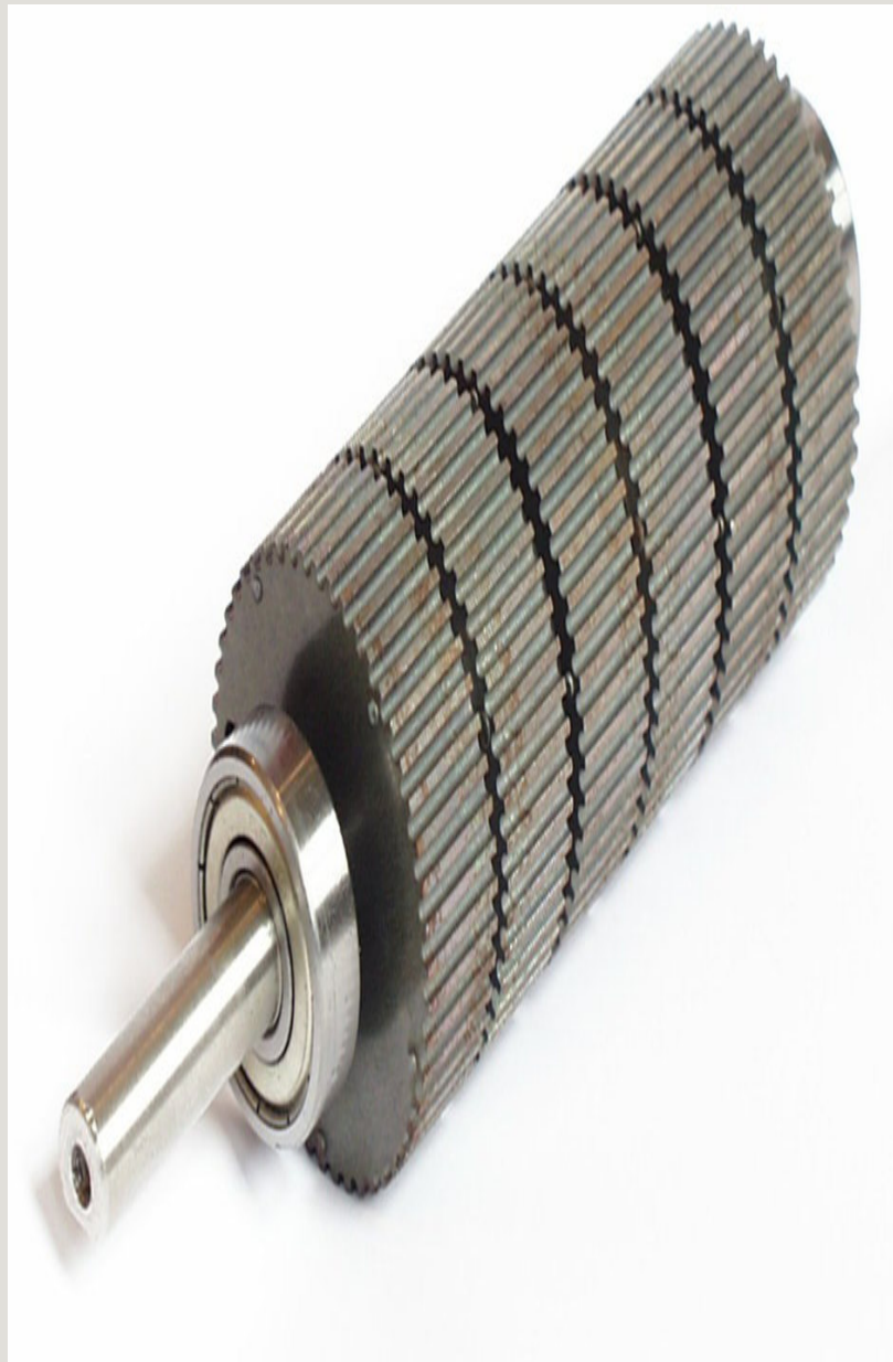
FIG. 10.7 Rotor of size 34 (3.4 in. or 8 cm diameter) 3-stack hybrid 1.8° stepping motor. The dimensions of the rotor end-caps and the associated axially-magnetised permanent magnet are optimised for the single-stack version. Extra torque is obtained by adding a second or third stack, the stator simply being stretched to accommodate the longer rotor.
