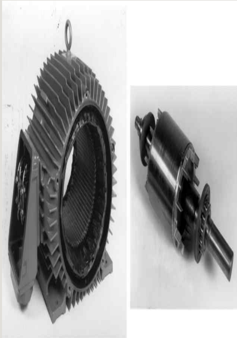
FIG. 5.12 Cage rotor for induction motor. The rotor conductor bars and end rings are cast in aluminium, and the blades attached to the end rings serve as a fan for circulating internal air. An external fan will be mounted on the nondrive end to cool the finned stator casing (as shown in Fig. 8.4).
