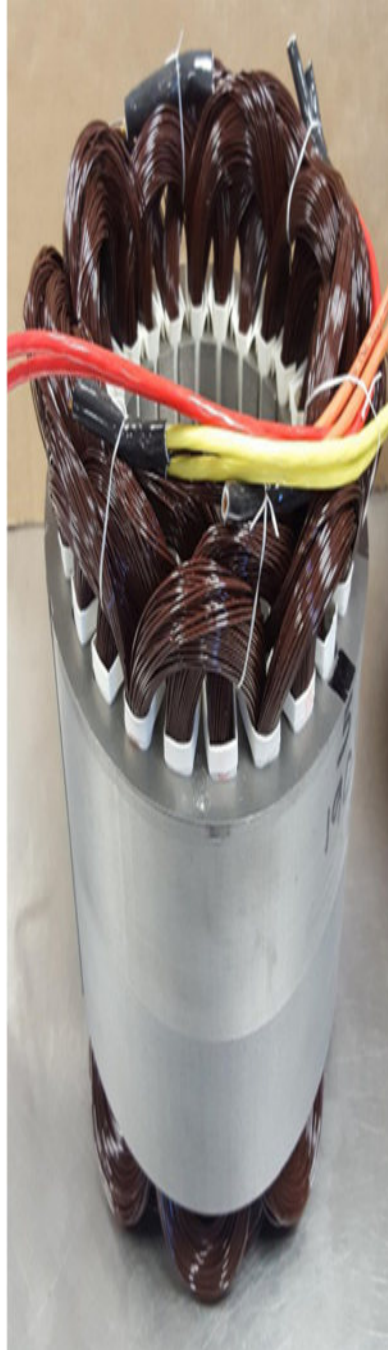
FIG. 5.6 The photo (left) shows the slotted stator core and slot liners, with the first of the three phase windings inserted. It is an eight-pole fully pitched two-layer winding, and we can see that one coil-side is in the top of a slot and the return side is in the bottom. The photo (right) shows the same motor with
