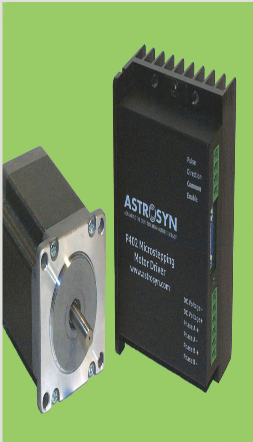
FIG. 10.19 Bipolar drive with integral heatsink providing a range of step divisions up to 25,600 steps/rev. It allows drive current to be set from 0.25 A to 2.0 A with supply voltage from
