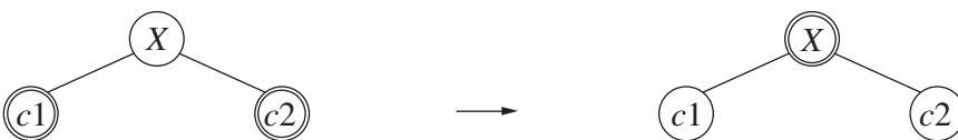
Figure 12.11 Color flip: Only if X 's parent is red do we continue with a rotation
