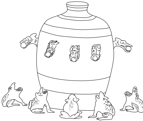
FIGURE 1.3 Schematic diagram of the world's first seismograph, invented in China in A.D. 132.
