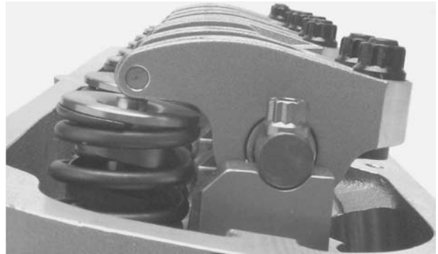
Figure 10.21 Type V push rod rocker arm with roller follower. (Courtesy Jesel Valve train Components.)
