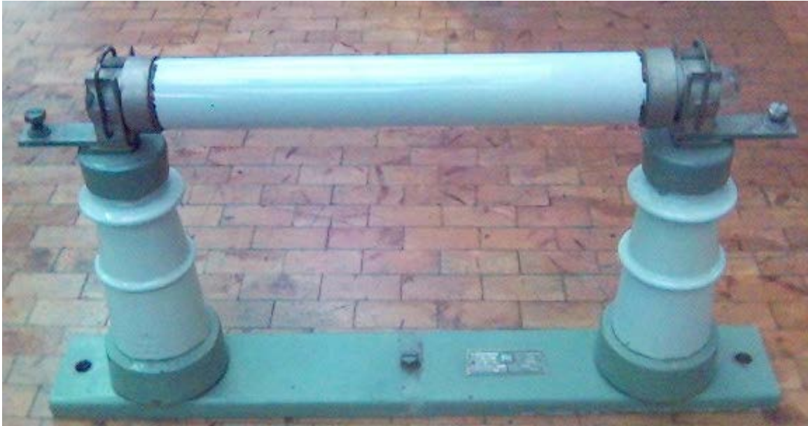
Older medium-voltage fuse for a 20 kV network
