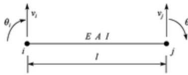
Fig. 8.5 Two-dimensional beam element with 2 nodes and 4 DOFs
