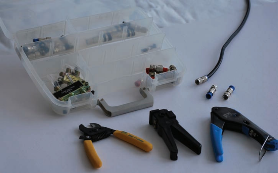
FIGURE 11-4 Coaxial cable with a connector, tools including a crimper, and an assortment of fittings.
