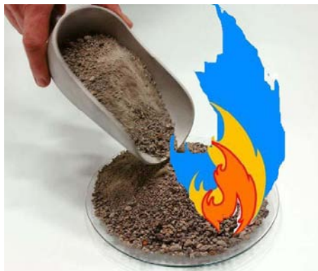
Figure 3.3 Combustible dust is made of fine particles that are easily ignited.
