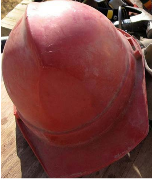
Figure 10.5 Damaged hardhats need to be discarded and replaced.
