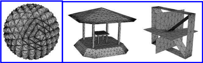
FIGURE 11.13: Several meshes produced with DIR3. In each case, small input angles requiring a collar region lead to the most mesh refinement.
