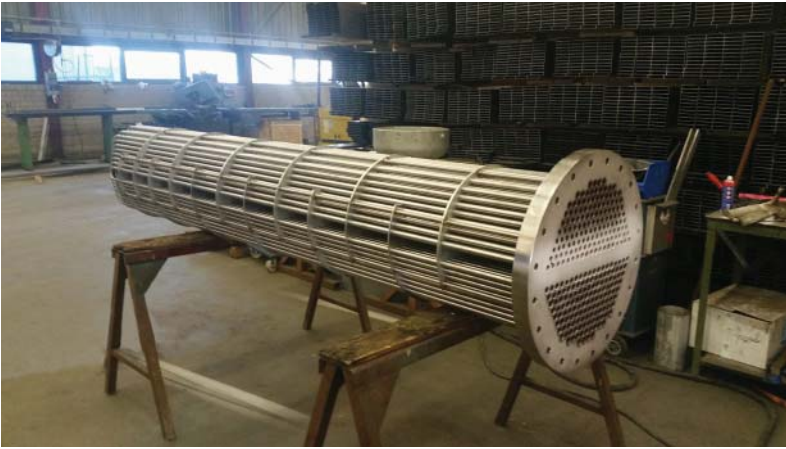
Figure 10.6 Surface heat exchanger.
