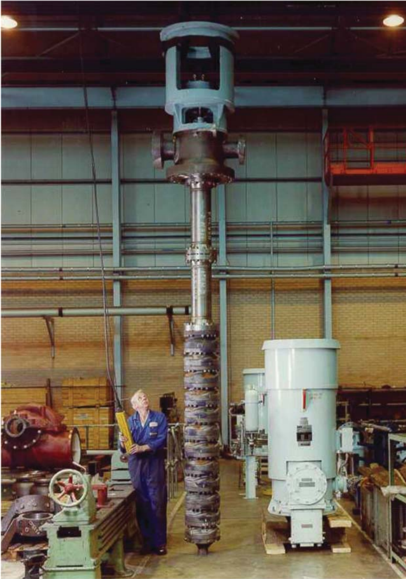
Figure 3.145 Multi cell submersible pump. Source: Sulzer.
