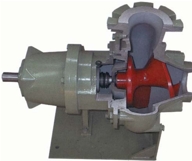
Figure 3.88 Francis vane pump. Source: Hus.
