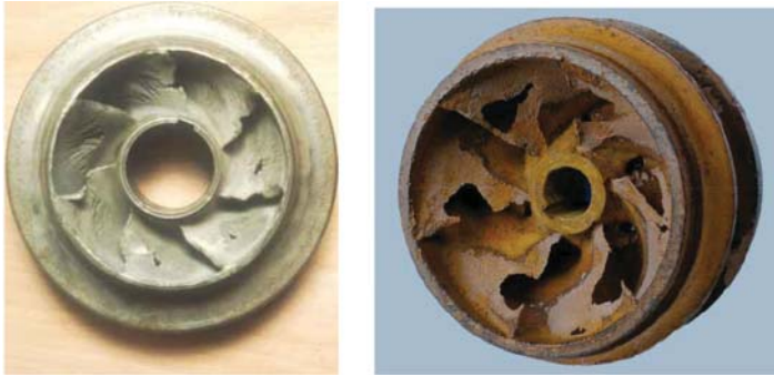
Figure 3.117 Attacked rotor centrifugal pump by cavitation. Source: Utwente.
