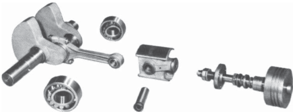
Figure 7.3 Components of compressor with cross head.
