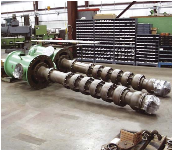
Figure 3.143 Multi cells submersible pump. Source: Sulzer Photo Gallery.
