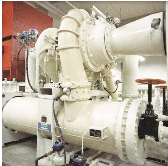
Figure 9.32 Two stage centrifugal compressor with intercooling. Source: Atlas Copco.
