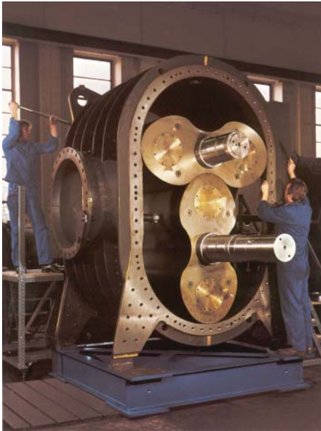
Figure 8.1 Operation principle roots compressor. Source: Howden.
