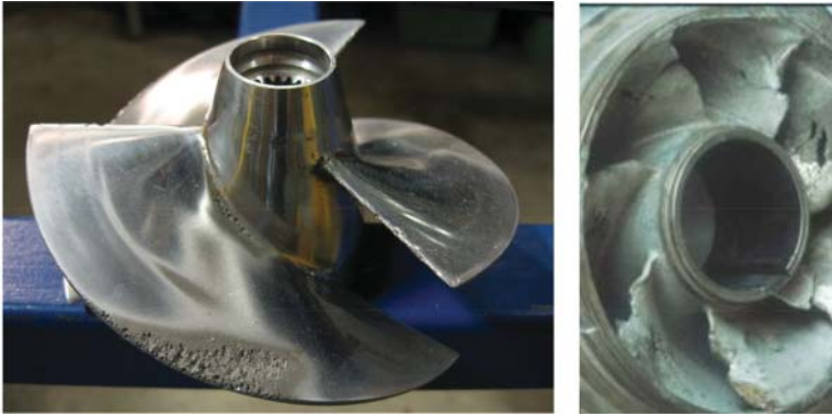
Figure 3.118 Axial pump damaged by cavitation. Source: Wikipedia and Utwente.
