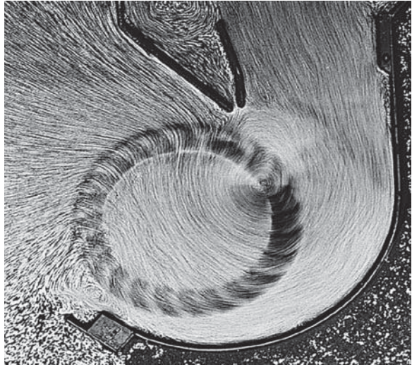
Figure 9.20 Cross-stream fan vortex. Source: Ebm-Papst.
