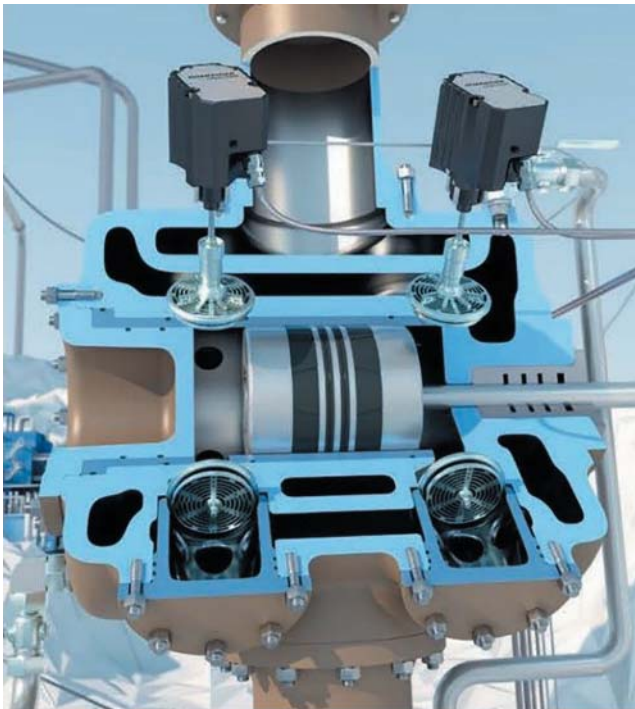
Figure 7.12 Valves double-acting piston. Source: Hoerlinger.
