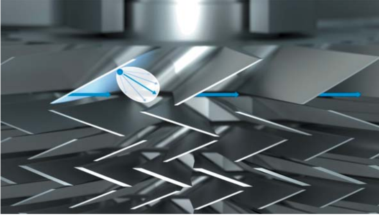
Figure 11.53 Principle of a molecular pump. Source: Pfeiffer.
