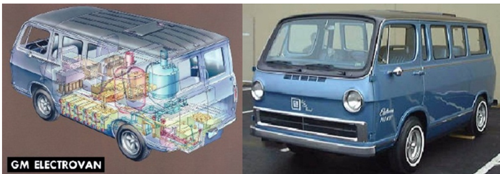
Figure 21. GM ElectroVAN, the first hydrogen fuel cell powered car introduced at 1966. The hydrogen and oxygen stored in super-cooled liquid in cryogenic tank.
