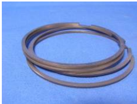
Figure 19. Prototype E2: 77 (Ti,Mo) (C,N)–20Ni–3 Mo
