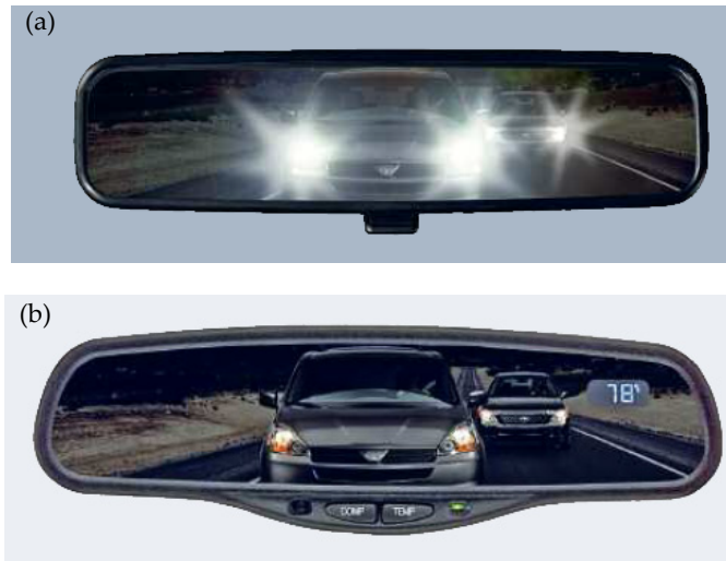
Figure 33. The conventional mirrors (a) and modern anti-glare rear mirrors for cars (b).
