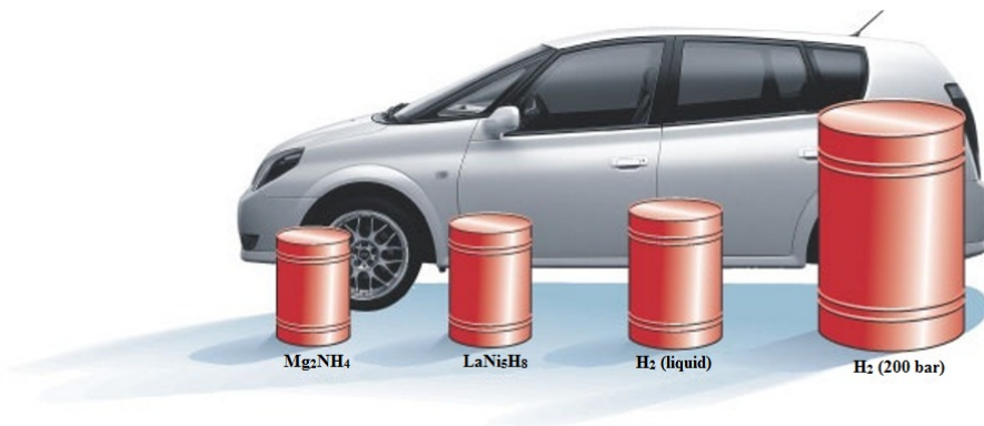
Figure 22. Comparison of volumetric density of different systems to store hydrogen (Schlapbach & Zuttel, 2001)
