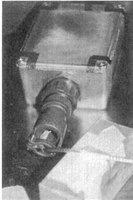
FIGURE 7.79 MIL-38999 connector measurement jig with lid fastened.
