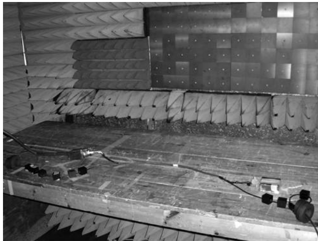
FIGURE 7.52 Photo of the cable under test with copper box on either end and copper tube and injection cable with ferrites.
