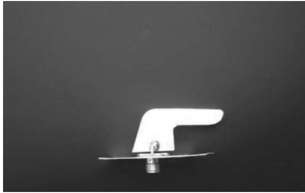
FIGURE 10.12 Blade antenna 10.8–17.4 GHz. (From Weston, D.A., Antenna to antenna coupling on an aircraft using a 1/10th scale model with results compared to the FEKO electromagnetic analysis program, EMC Europe , Wroclaw, Poland. © 2010, IEEE.)
