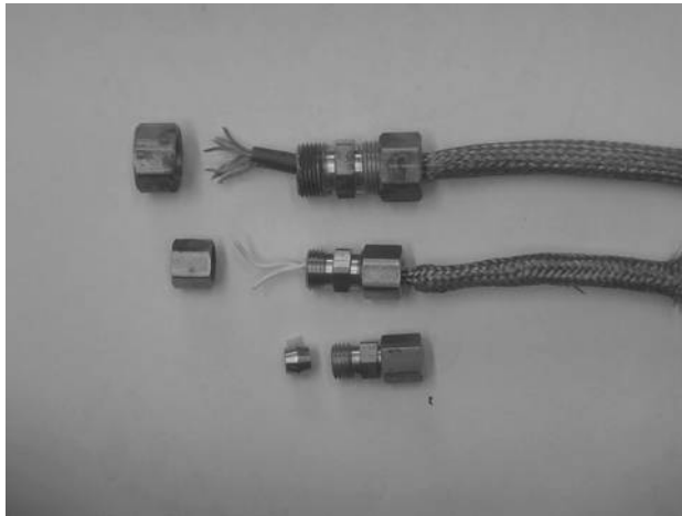
FIGURE 7.163 Photo of plumbing fittings used for shield termination.
