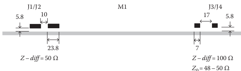
FIGURE 11.13 Microstrip 1 dimensions and impedances.
