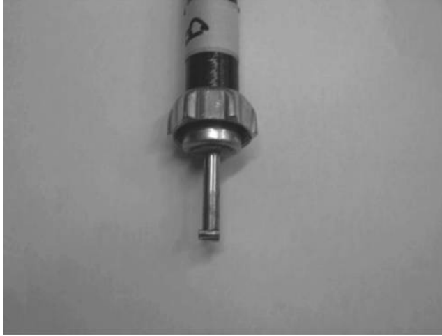
FIGURE 7.36 Photo of the rod centered in conduit forming a 50 \Omega coaxial cable.
