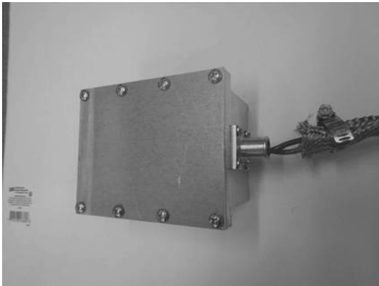
FIGURE 7.161 Braid connected with a hose clamp to a nipple mounted on the enclosure.
