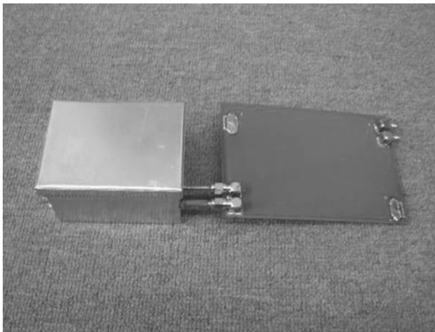
FIGURE 11.4 Overall stripline PCB and enclosure with limited shielded connectors and loads.
