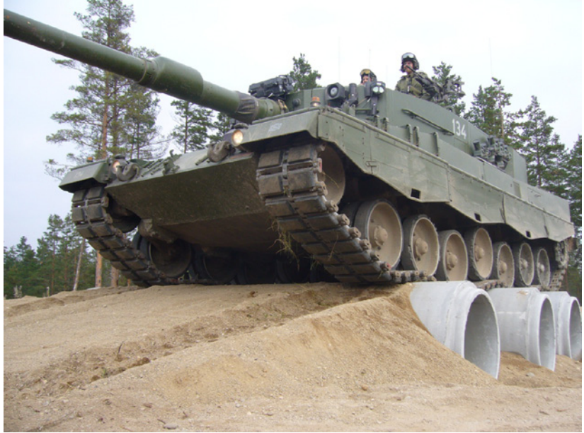
Figure 3.24 Unsurpassed strength of concrete pipes demonstrated above. Reproduced by permission of Basal AS.
