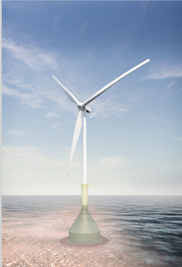
Figure 3.31 Concrete Gravity Base solutions are being developed for water depths in excess of 20m to support turbines of 5MW and greater. These structures will be manufactured in serial production facilities, floated to site, and then sunk and ballasted. Reproduced by permission of Gravitass.
