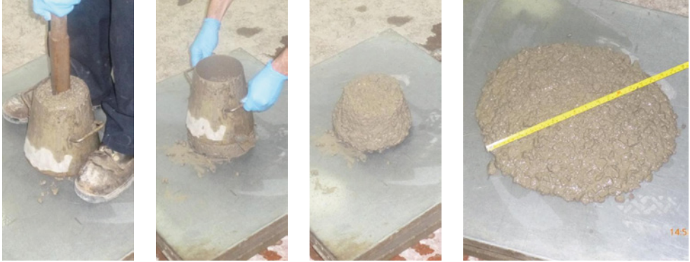
Figure 4.16 A flowability test (diameter of spread) rather than a slump test (height of slump) is used for Self Compacting Concrete. Reproduced by permission of BASF Plc.
