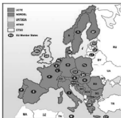
Figure 2.34 Synchronous regions in the European area. Source UCTE system adequacy forecast 2005–2015. Reproduced with permission. The UCTE region is divided as shown. Western Ukraine is also synchronous with UCTE
