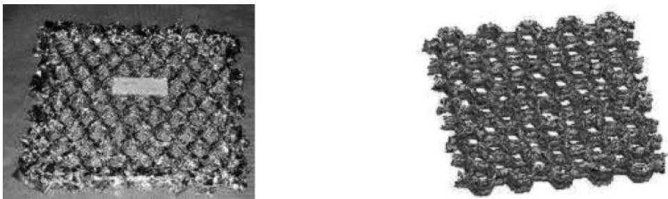
Figure 11.3 Crushing of honeycomb, test and simulation.
