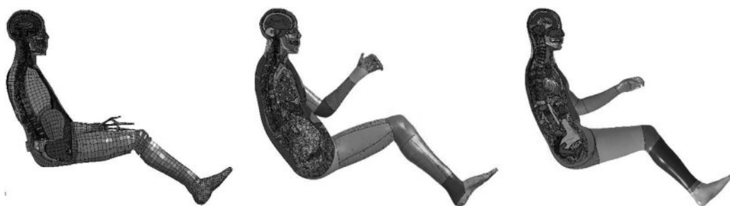
Figure 14.4 Mid-size male models, cut in the sagittal plane to visualize the internal structures: THUMS v3 (TMC 2008), THUMS v4 (Watanabe et al 2011), GHBM (Vavalle et al 2013).
