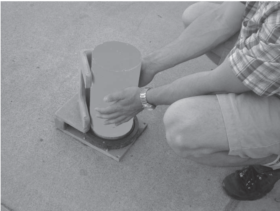
FIGURE A.40 Capping a concrete cylinder using an alignment device.
