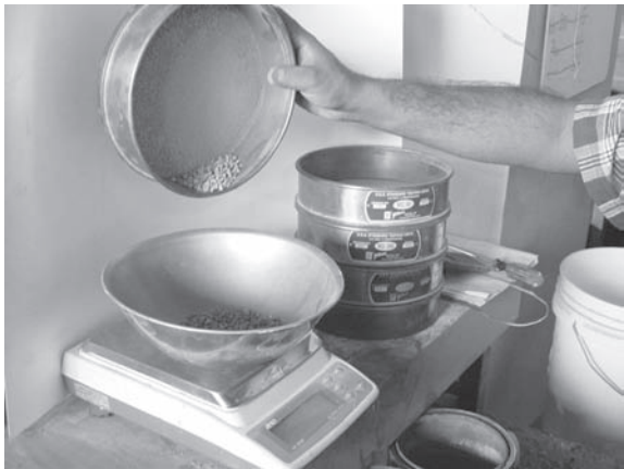
FIGURE A.23 Weighing aggregate retained in sieves.
