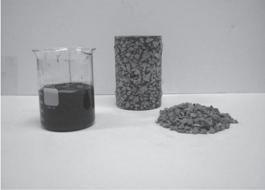
FIGURE 9.3 Photo showing asphalt cement, aggregate, and asphalt concrete. (Courtesy of FHWA)
