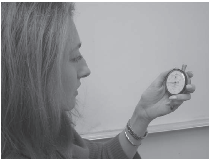
FIGURE A.1 Examining the sensitivity and range of a dial gauge.
