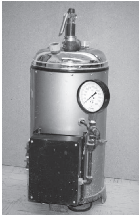
FIGURE 6.7 Cement autoclave expansion apparatus. (Courtesy of Humboldt Mfg. Co.)
