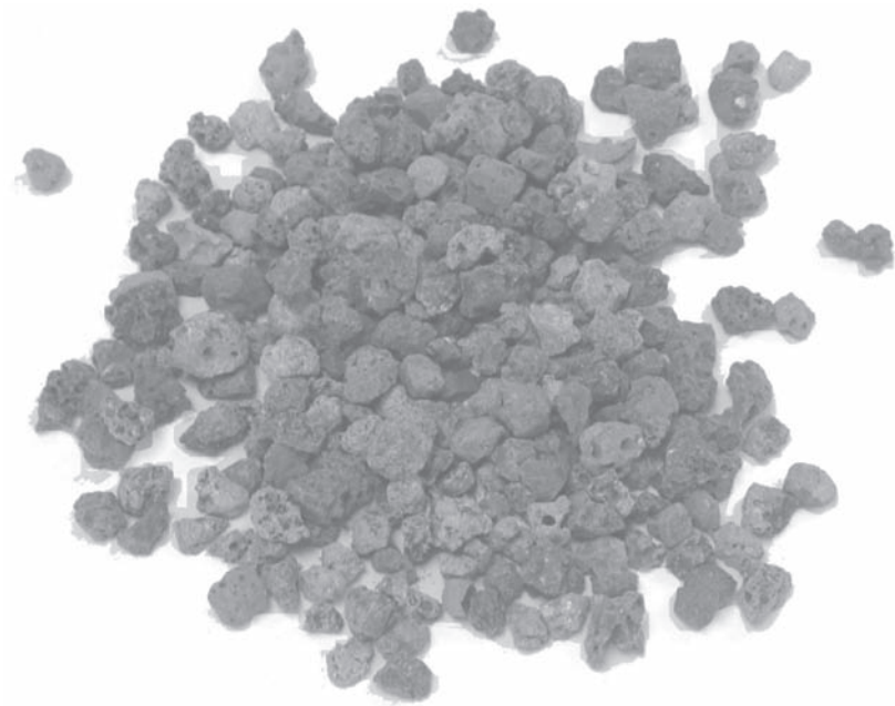
FIGURE 7.48 Aggregate used for lightweight concrete.
