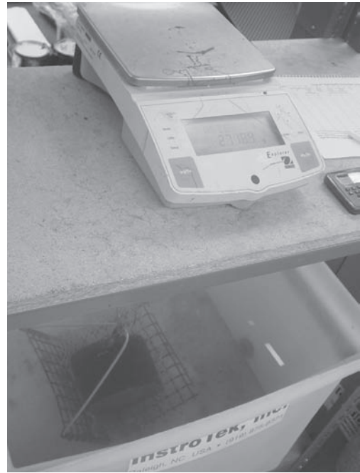
FIGURE A.65 Weighing HMA specimen in water.
