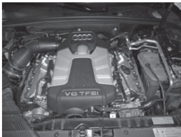
Figure 9-14 The Audi supercharged V6 that is used in the Porsche® Cayenne®, Porsche® Panamera®, and Volkswagen Touareg hybrids.
