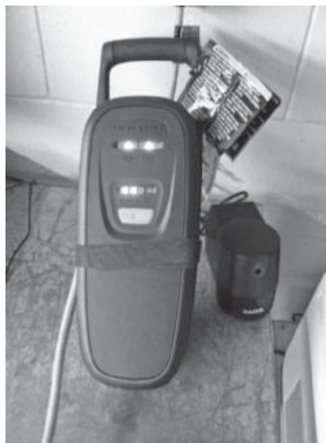
Figure 6-25 The charging unit has a series of lights that indicate the charging status.
