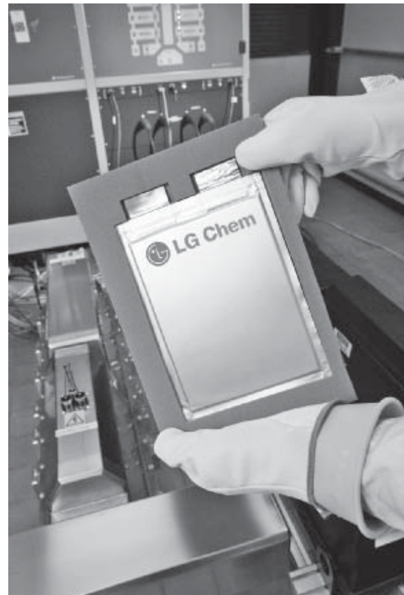
Figure 6-23 The Volt's battery pack consists of 288 of these Li-Ion cells.
