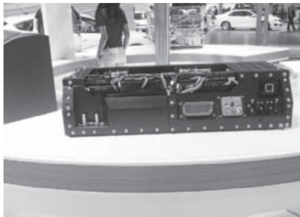
Figure 5-40 The battery pack in a Ford Focus BEV.
