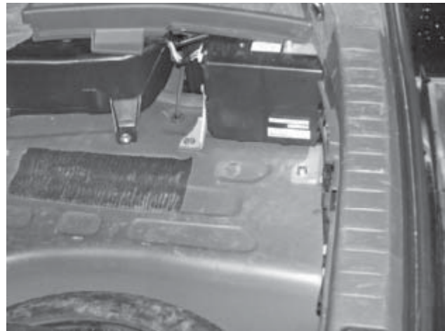
Figure 10-20 Note that the auxiliary battery is tucked into the corner of this trunk.
