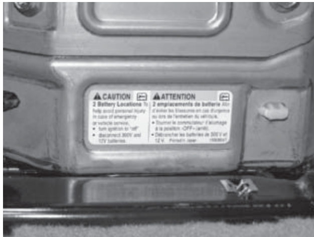
Figure 10-19 This warning label states that there are two separate batteries.
