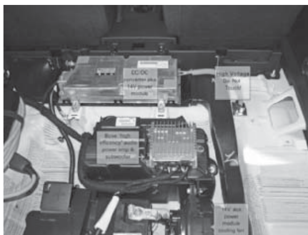
Figure 6-21 The various components in the luggage compartment of a Volt.
