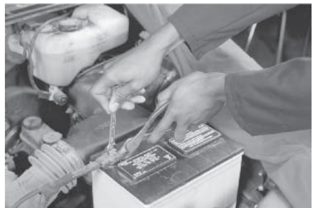
Figure 4-29 When working on a battery or when disconnecting it, always disconnect the negative cable first.
