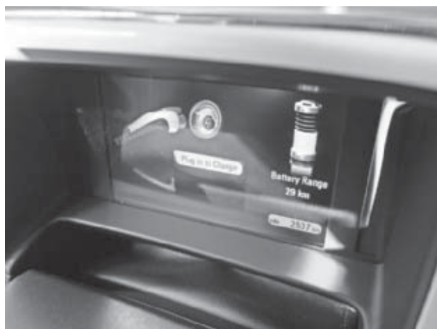
Figure 6-27 An example of the charging status as displayed on the center stack.
