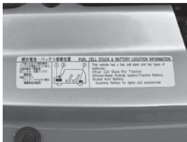
Figure 11-19 The sticker says this vehicle is a fuel cell hybrid vehicle and defines the purpose of the major components.
