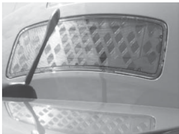
Figure 5-29 The solar panel built into the spoiler on some models of the Leaf.
