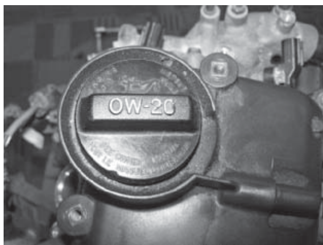
Figure 10-30 Many hybrids require very light engine oil.
