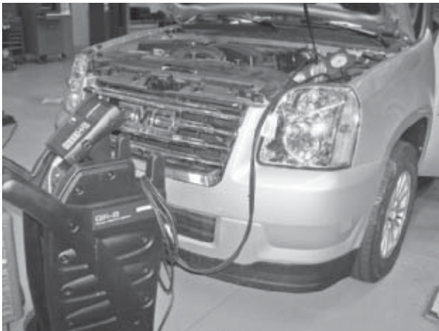
Figure 4-8 A smart charger connected to the battery of a GM two-mode hybrid vehicle.
