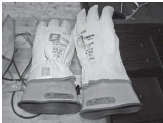
Figure 10-5 A pair of lineman’s gloves covered with leather work gloves.
