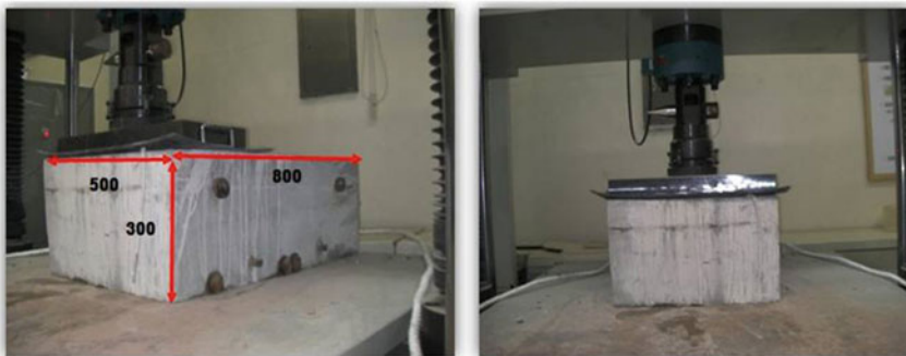
Fig. 23.4 Compressive strength Load Test
