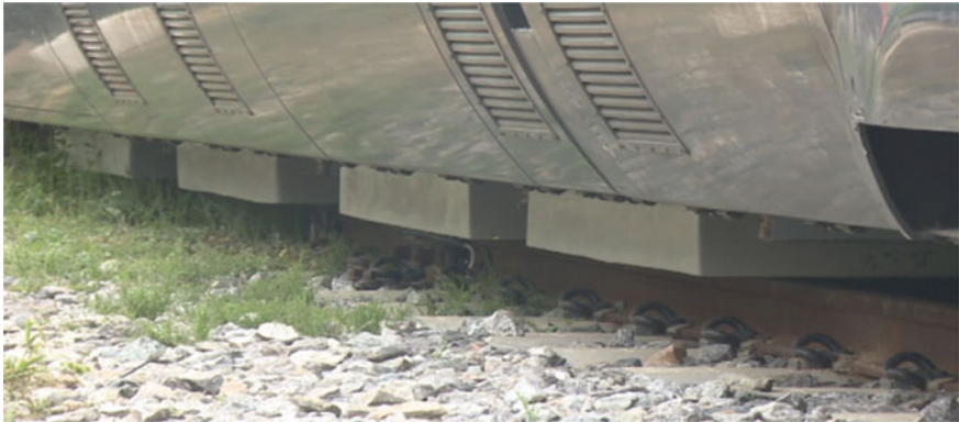
Fig. 17.11 Photograph of installed four pickup units
