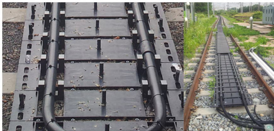
Fig. 17.8 Photographs of developed 128-m transmitter track
