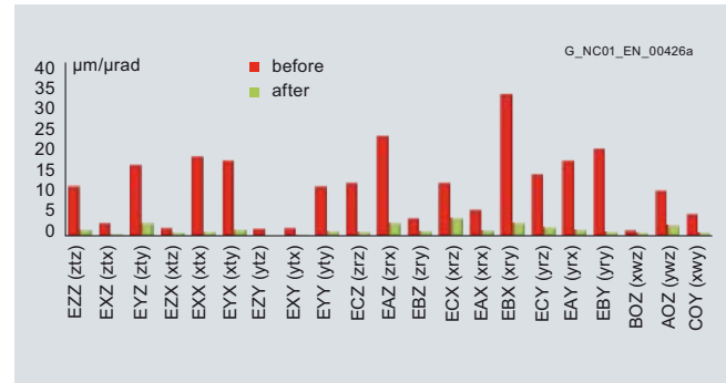
Comparison of kinematic single errors (according to ISO 230) of an uncompensated and a compensated machine (ETALON compensation data and VCS application)
