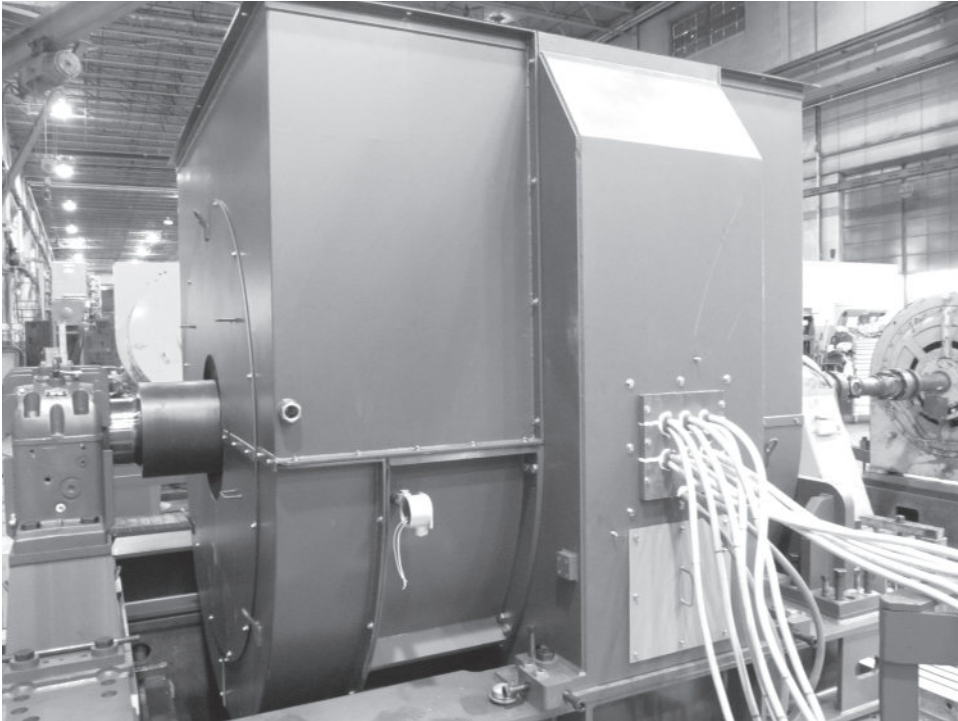
FIGURE 17-1 Synchronous motor under construction.
