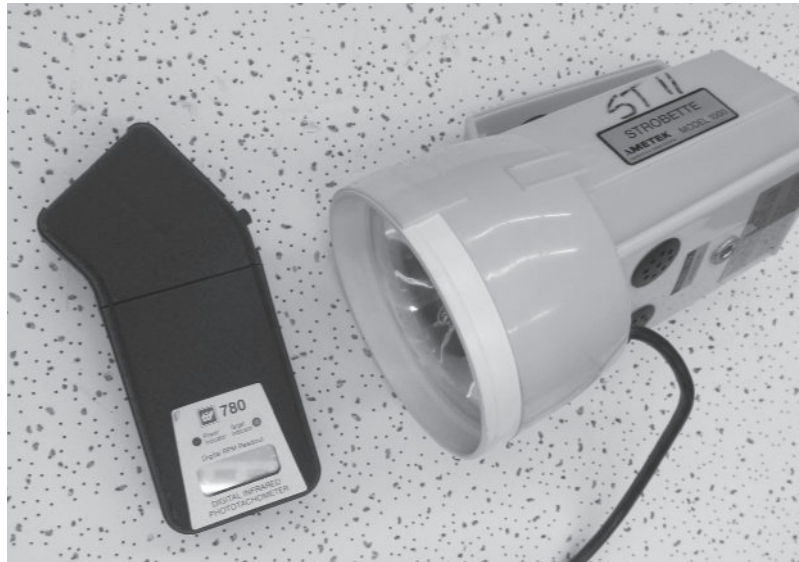
FIGURE 25-5 A strobe tachometer and a photoreflective tachometer.
