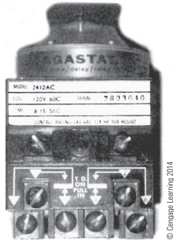
FIGURE 10-10 Mechanical timer uses air (pneumatic) timing.
