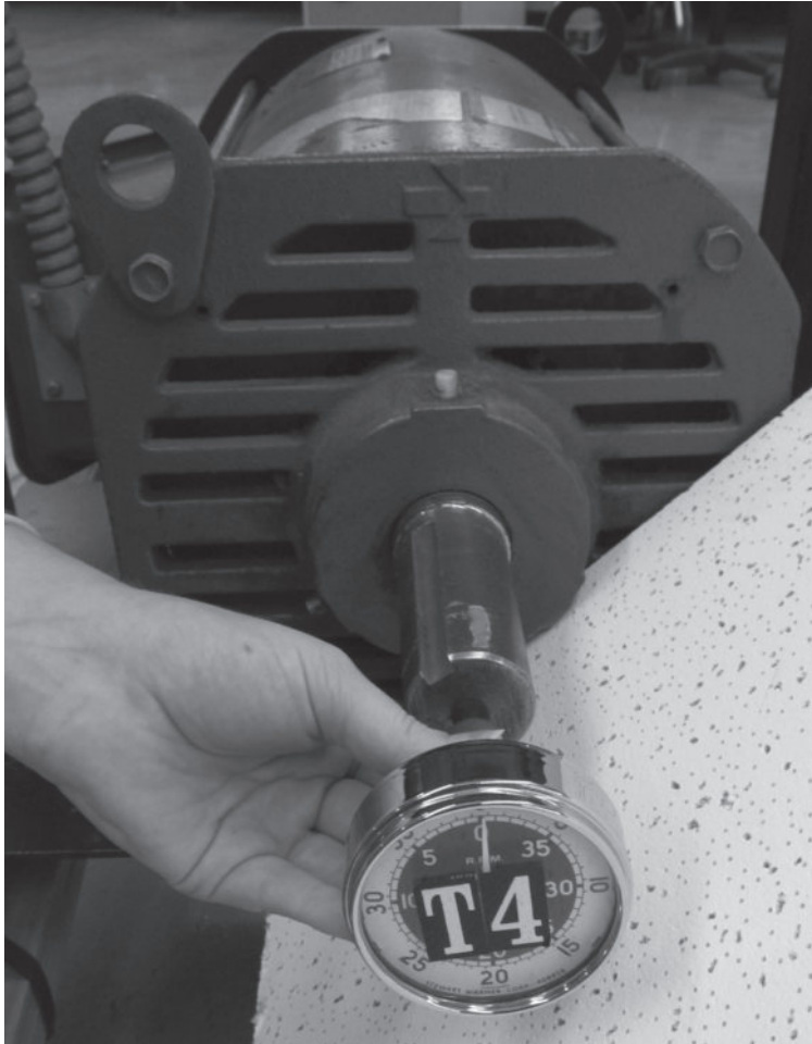
FIGURE 25-6 Mechanical tachometer used to measure shaft RPM.
