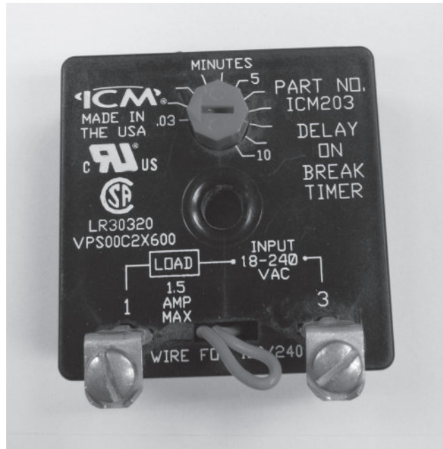
FIGURE 14–9 Small solid state timers can provide many functions such as “on-delay”.
