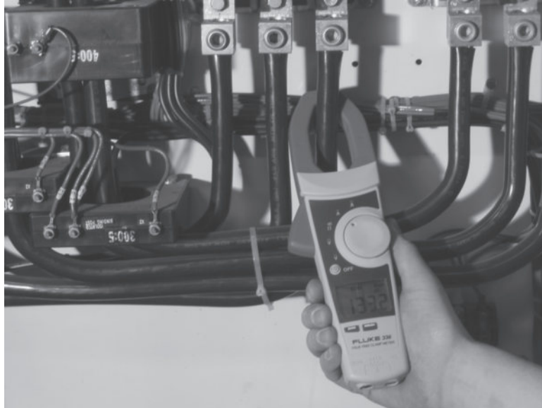
FIGURE 24-4 Use a clamp-on ammeter to test motor power system.
